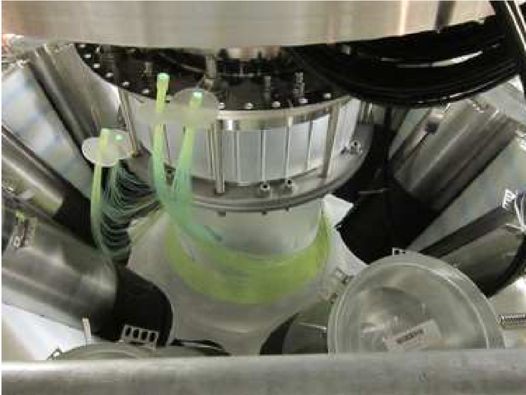
Figure 4.11: The neck region of DEAP, before installing the neck filler blocks, showing the wavelength shifting fibres wrapped around the bottom 10 cm of the neck. Image taken from [150].
