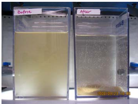
Figure 5: Picture of OSPW samples before and after coagulation-flocculation followed by sedimentation processes with 200 mg/L alum and 20 mg/L CTI TL.
