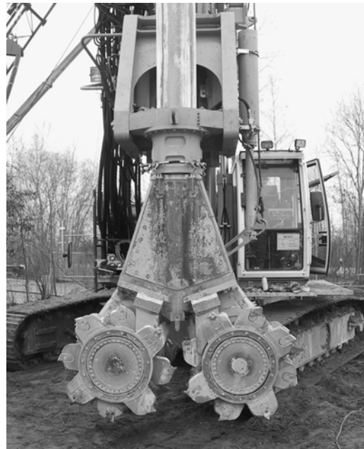
Figure 1. CSM head mounted to Kelly bar
