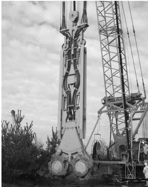
Figure 2. Wire rope-suspended CSM unit
