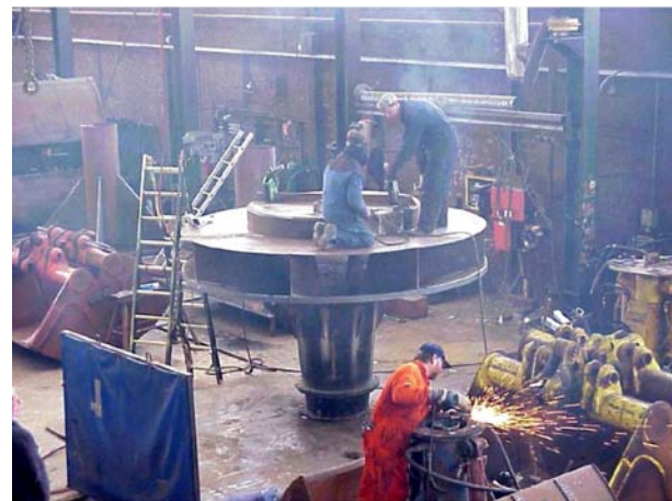
Figure 5. Tremie/Diffuser used at Lake Zevenhuizerplas shown upside down (from Mastbergen et al. 2004).
