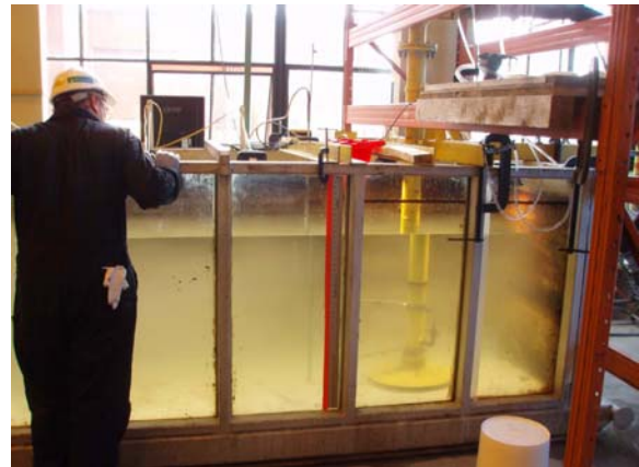
Figure 12. Experimental Flume with tremie/diffuser installed.
