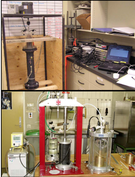
Figure 13. Deltares column settling and seepage induced consolidation testing equipment.
