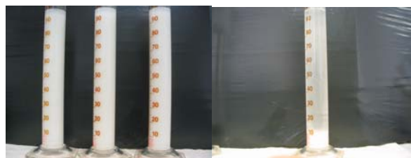
Figure 5. Comparison of supernatant clarity with PAMs of an anionic (left, 4, 10 and 20ppm) and a non-ionic (right 10ppm).
