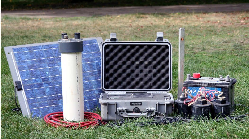
Figure 4-5. NIMS (Narod Intelligent Magnetotelluric System). From left to right: solar panel, fluxgate magnetometer (white cylinder), magnetometer cable (red), data logger (grey box), electrode wire (black), grounding stake, four lead chloride electrodes (black cylinders) and a car battery.
