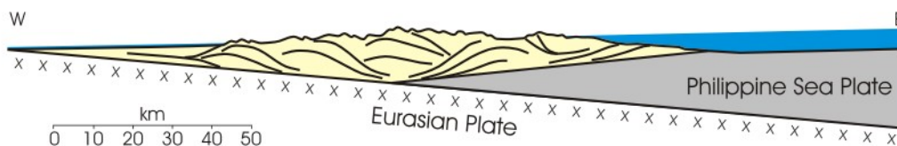
Figure 2-7. Simplified cross-section of the Taiwan orogen deformed via thin-skinned tectonics. Redrawn from Suppe, 1987.
