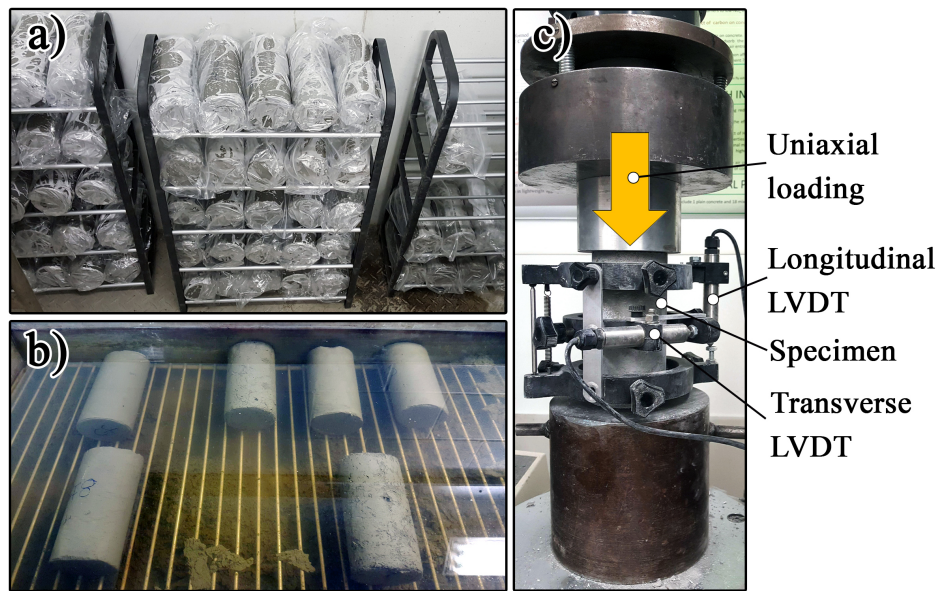
Fig. 6.1. Freeze-thaw test procedure: a) sealed specimens are freezing inside a walk-in freezer; b) thawing in temperature controlled water bath; and c) uniaxial compression test apparatus.
