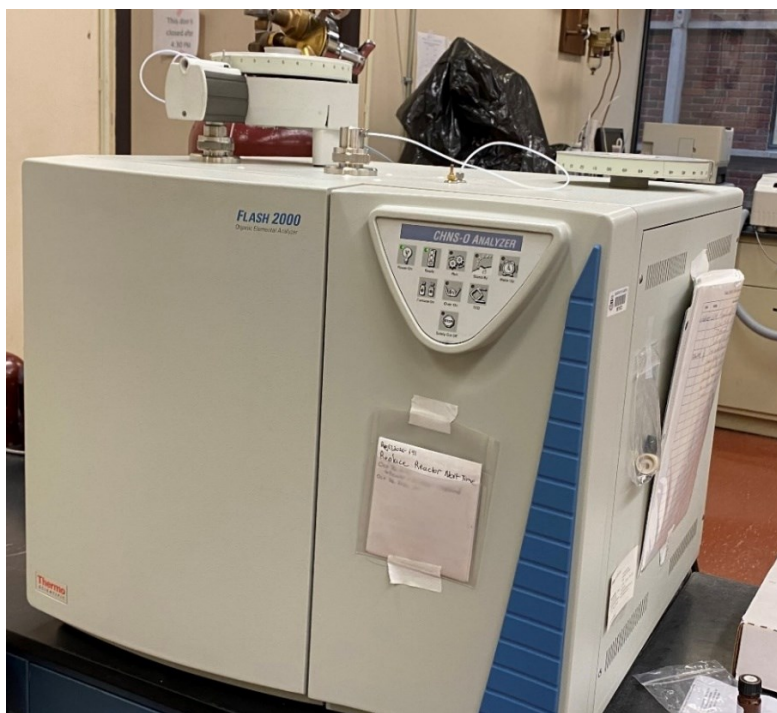
Figure 17: Thermo Fisher Flash 2000 Organic Elemental Analyzer used for CHNS analysis.
