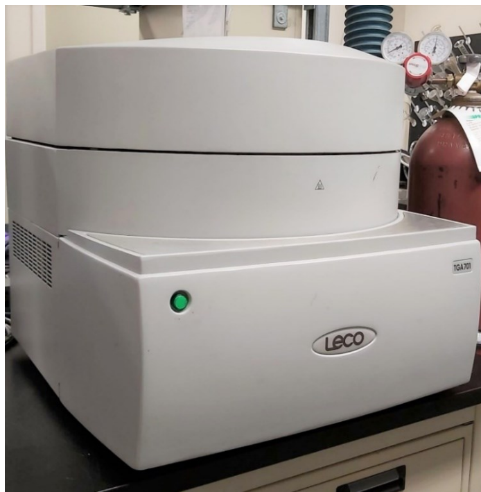
Figure 16: LECO TGA 701 used for Proximate analysis of Corn stover, Wheat straw and Hardwood.
