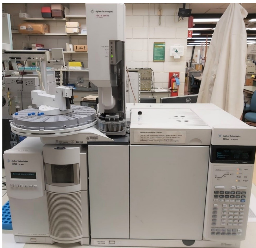
Figure 18: Agilent Technologies (GC 7890A – MS 5975C) used for GC-MS analysis of Heavy oil.
