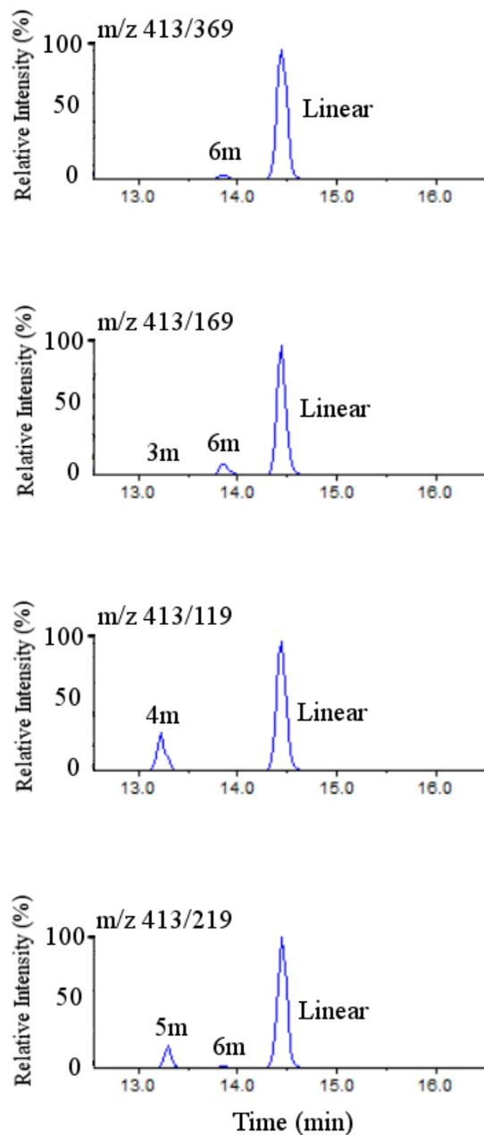
**Figure B-1.** Chromatogram of PFOA isomer profiles from standards, including mass transitions and relative intensity
