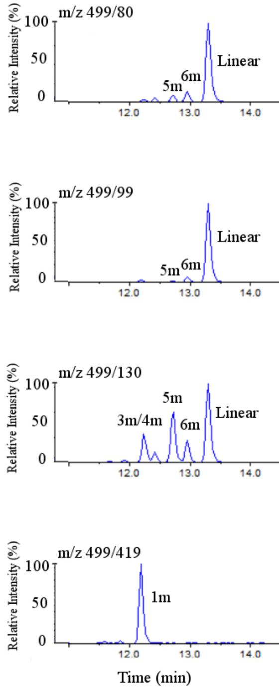
**Figure B-2.** Chromatogram of PFOS isomer profiles from standards, including mass transitions and relative intensity
