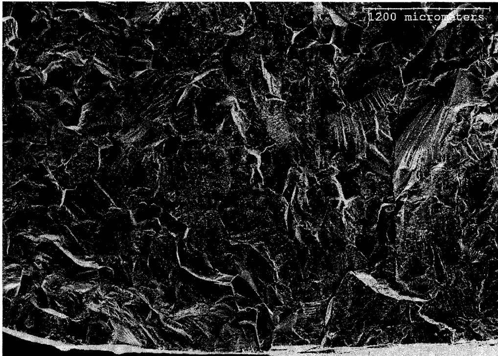
Figure 72: SEM Image of Alloy 3 Fracture Surface (4-hour cooled) (SE)
