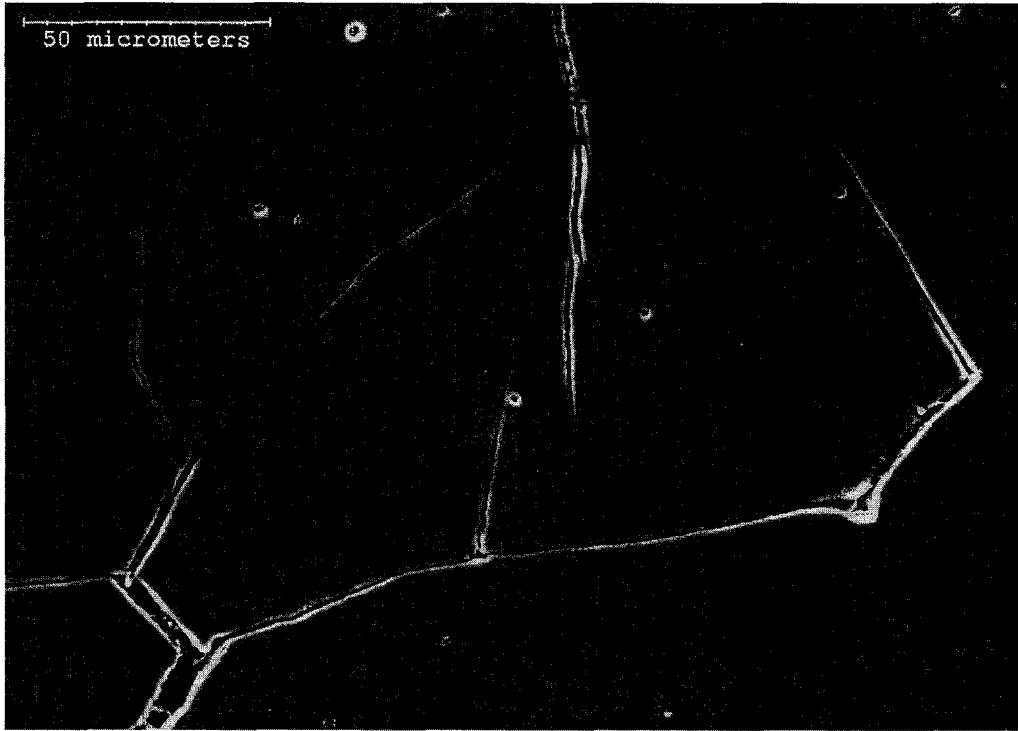
Figure 63: SEM Image of Alloy 2, 520 MPa Compression (air cooled) (SE, polished)
