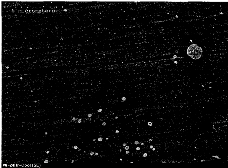
Figure 45: SEM Image of Alloy 8 Homogenized and 24-hour Cooled (SE)
