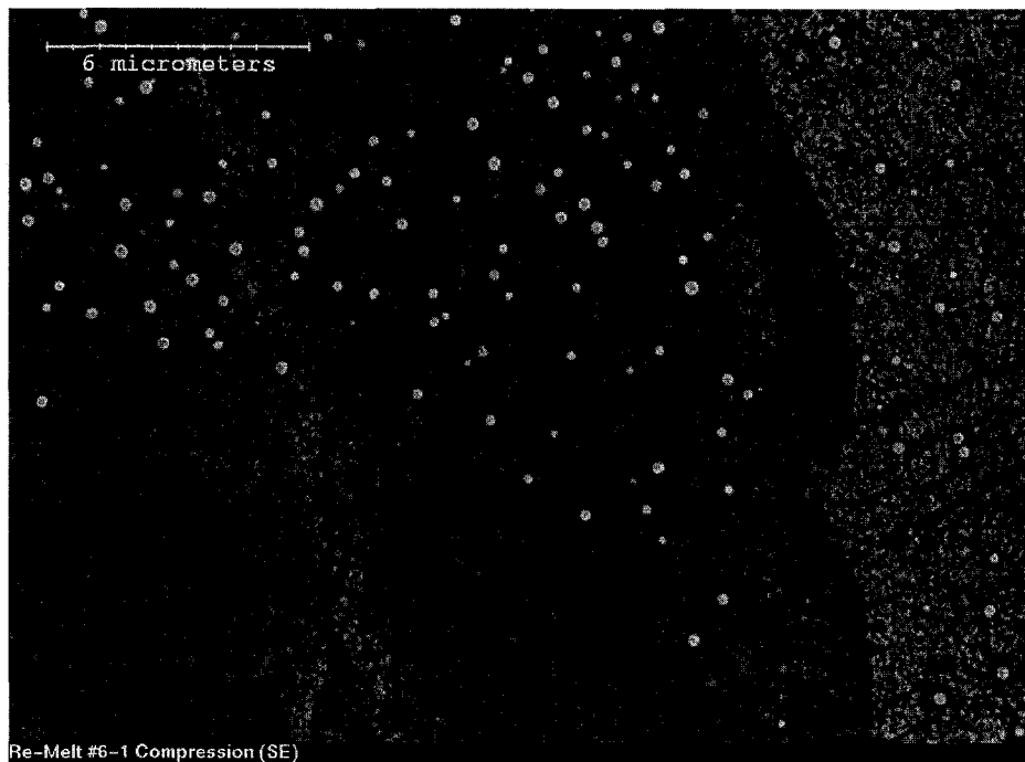
Figure 40: SEM Image of Alloy 6 Homogenized and Air Cooled (SE)
