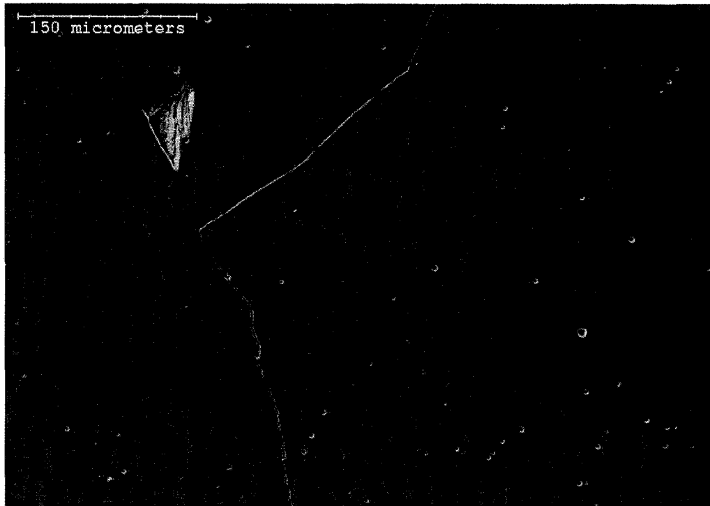
Figure 74: SEM Image of Alloy 3, 358 MPa Compression (4-hour cooled) (SE, polished)
