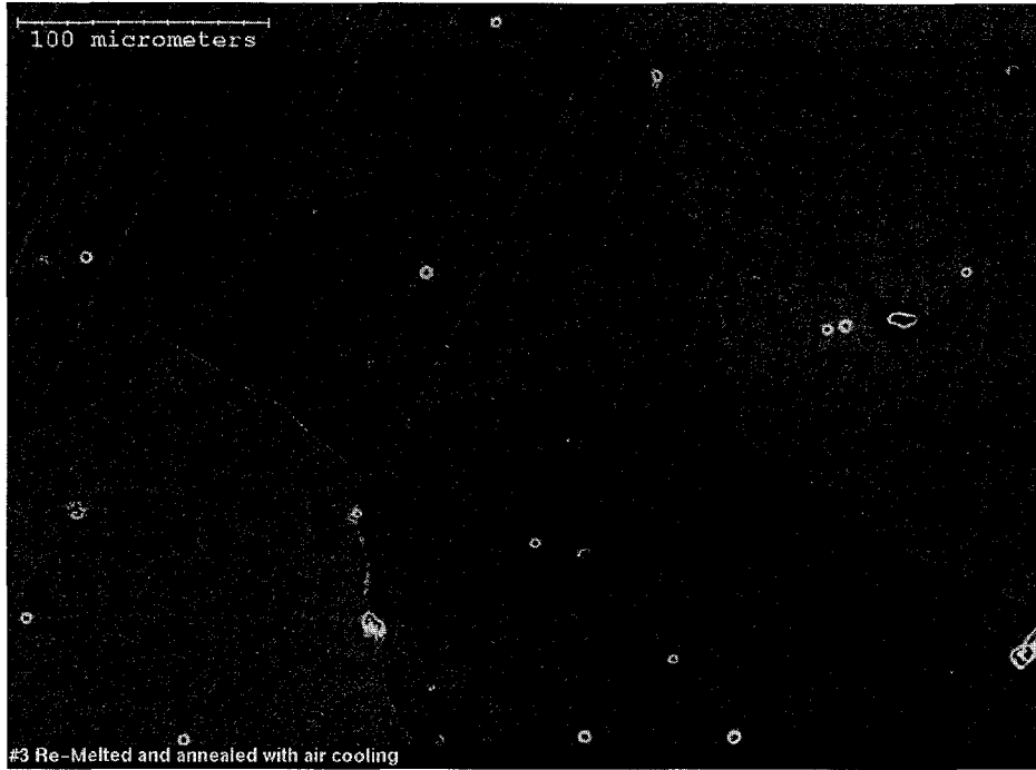
Figure 38: SEM Image of Alloy 3 Homogenized and Air Cooled (SE)
