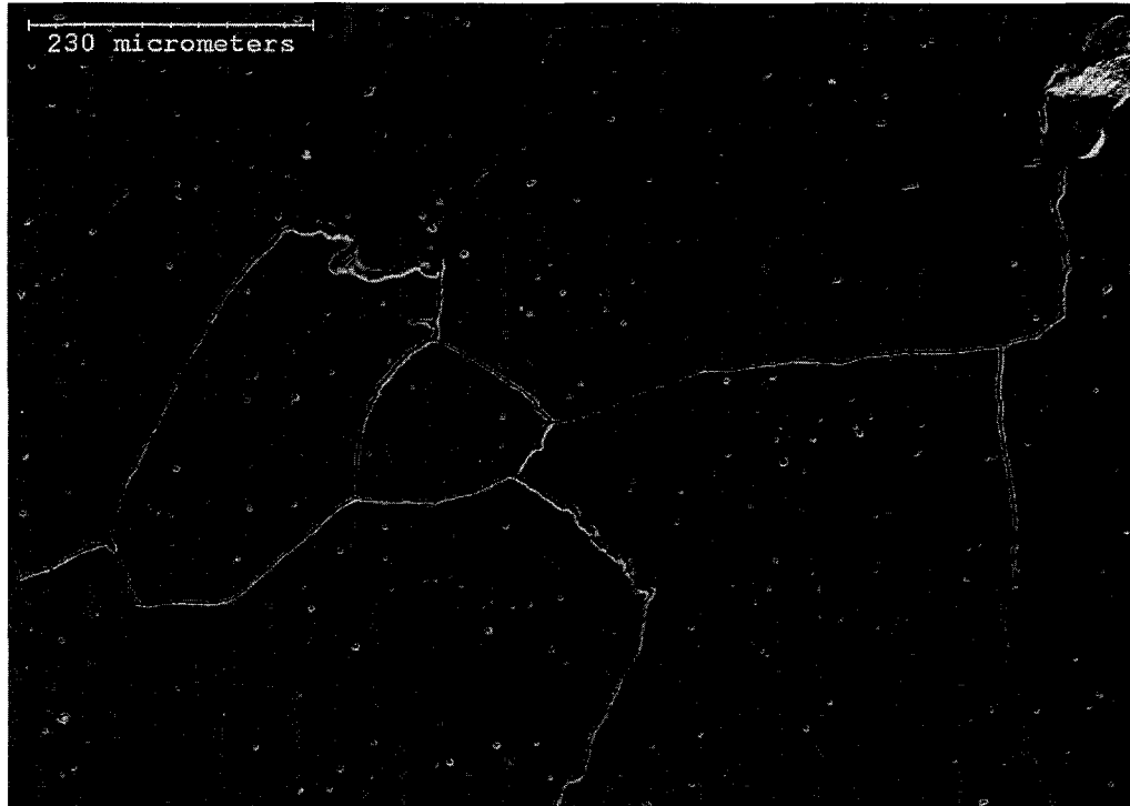
Figure 79: SEM Image of Alloy 6, 753 MPa Compression (air cooled) (SE, polished)
