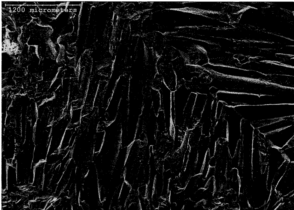
Figure 78: SEM Image of Alloy 6 Fracture Surface (24-hour cooled) (SE)
