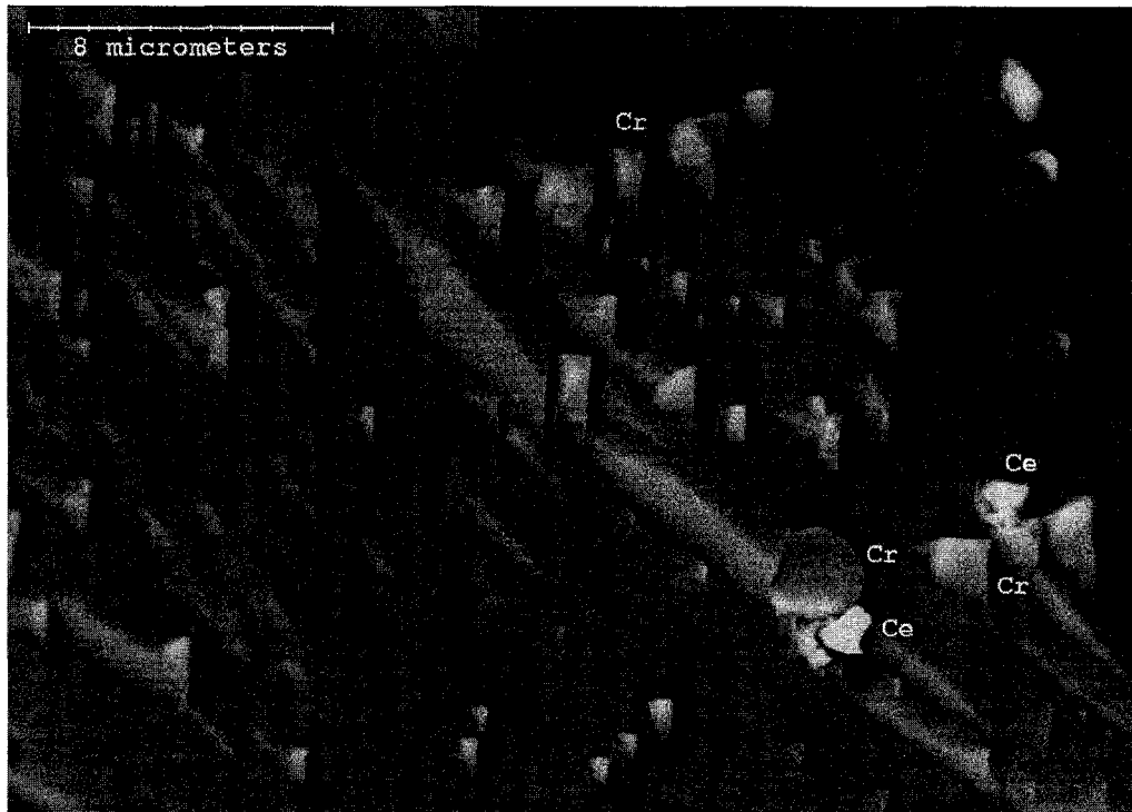
Figure 69: SEM Image of Alloy 2 Fracture Surface with Ceria and Chromium (4-hour cooled) (SE)
