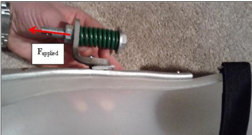
$F_{\text{applied}}$  was assumed to be 900N corresponding to the maximum force applied by the gas spring. Calculations were performed to ensure the cable anchor bracket was safe under bending due to the applied cable tension force.
