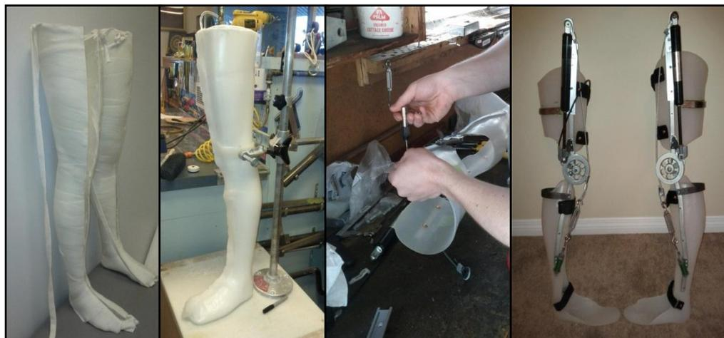
Selected steps of prototype manufacturing, from left to right: casts taken of the participant's legs, locating and drilling the knee center, fixing prototype component to the manufactured KAFO, two manufactured and assembled prototypes
