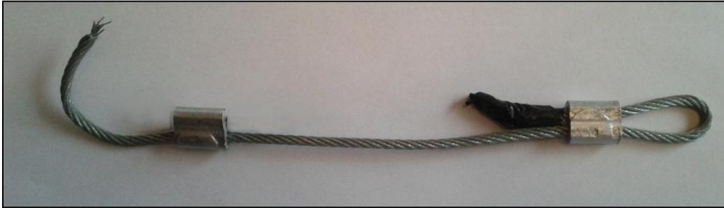
Failure in the dead end clamp allowed the cable to ‘pull-out’
