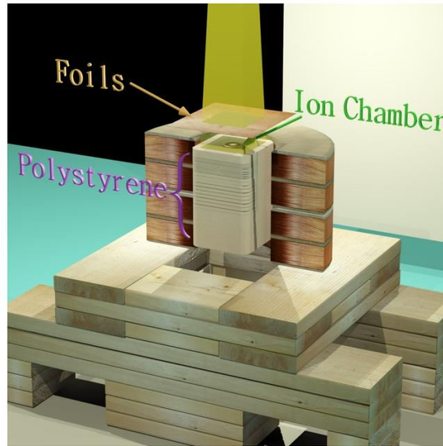
Figure 1: Surface dose was measured below copper and aluminum foils of various thicknesses. The foils were placed in the beam on top of the polystyrene phantom surface with an inset parallel plate ion chamber. Foils were in direct contact with the phantom surface (gap in image is introduced to show the ion chamber). The phantom was inside the bore of dual solenoid electromagnets positioned on top of a wooden support structure.
