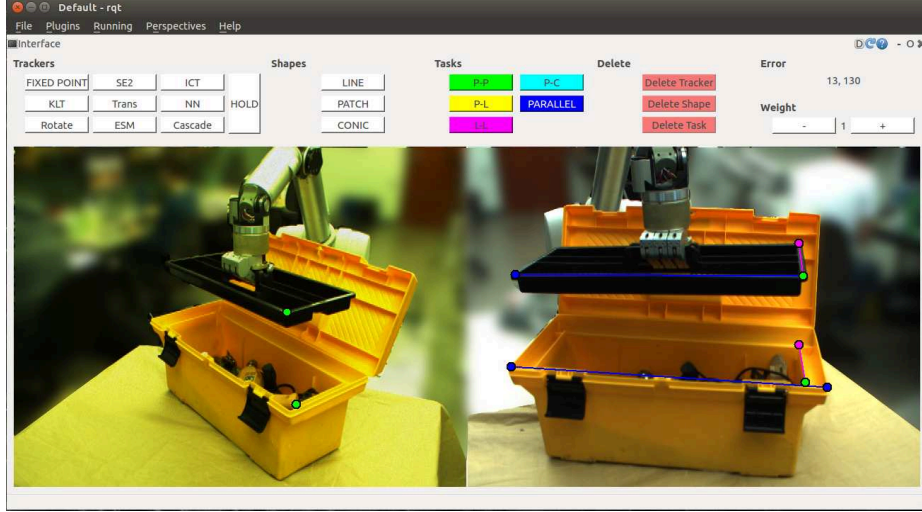
Figure 1.5: Using the Visual Task Specification Interface users are able to easily initialize trackers and define visual geometric constraints that help direct the robot to a given goal.
