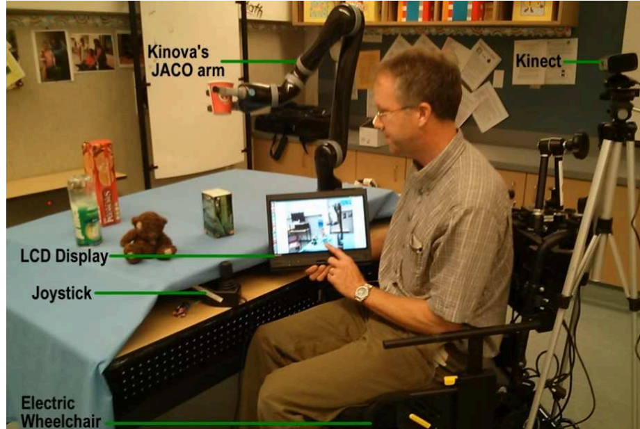
Figure 1.2: Vision-based User Interface to a 6DOF robot arm and hand. By pointing and selecting in a 2D video image of the scene, the user can point to objects, select grasp types and execute robot actions.
