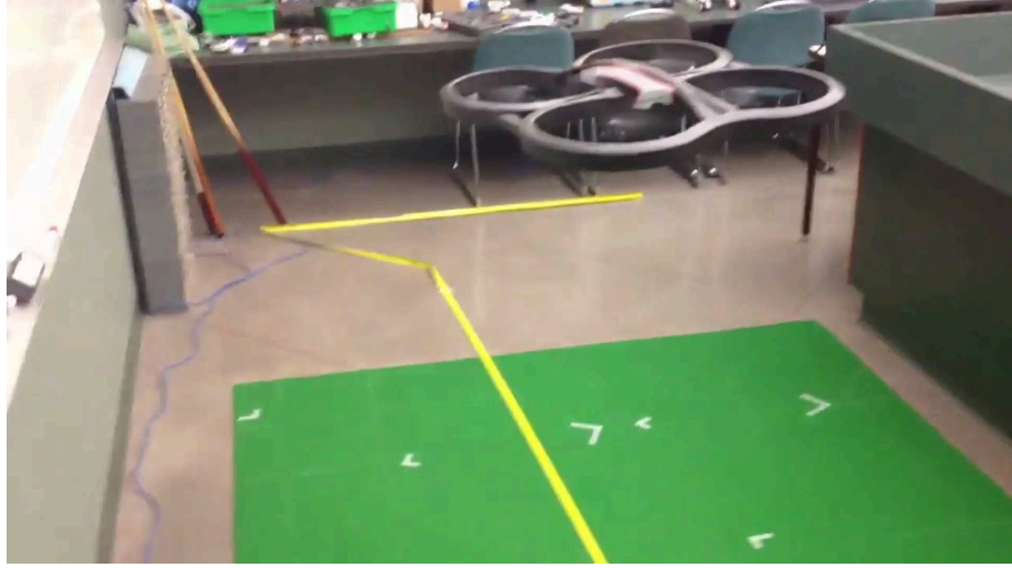
Figure 4.9: Line alignment with UVS controlling the drone’s yaw position. Once UVS is active users manually control roll and pitch to position the drone accordingly.
