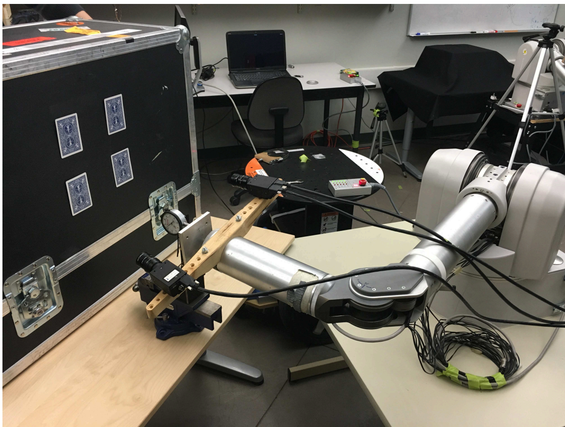
Figure 5.14: Robot repeatability for 4 DOF robot with eye-in-hand camera configuration
