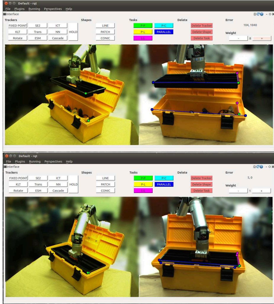
Figure 4.5: Top: User defines geometric constraints visually. Green points indicate point-to-point constraints. Magenta indicates a line-to-line constraint, and finally blue is used for parallel constraints. Bottom: Once the constraints have been specified the Visual Servoing takes place minimizing the error of the defined goals.
