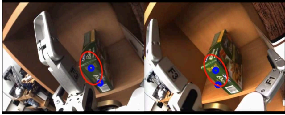
Figure 4.8: Grasping done via Uncalibrated Visual Servoing. A colour tracker is initialized to track the position of the green box. A target is defined in between the hand’s fingers. Once a threshold is reached the hand closes completing the grasp.
