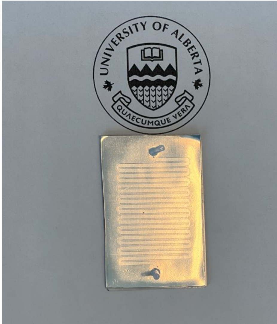
Figure A2. shows a microfluidic device microfluidic device with an incorporated metalized sheet.
