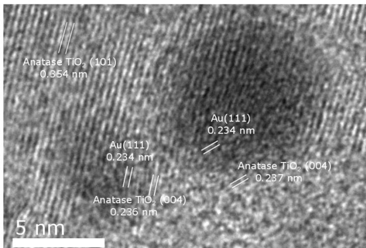
**Figure 5.** HRTEM image of Au-TiO<sub>2</sub> interface illustrating the coherent heterointerface between Au (111) and TiO<sub>2</sub> (004) that support the Au NPs in the TiO<sub>2</sub> lattice.
