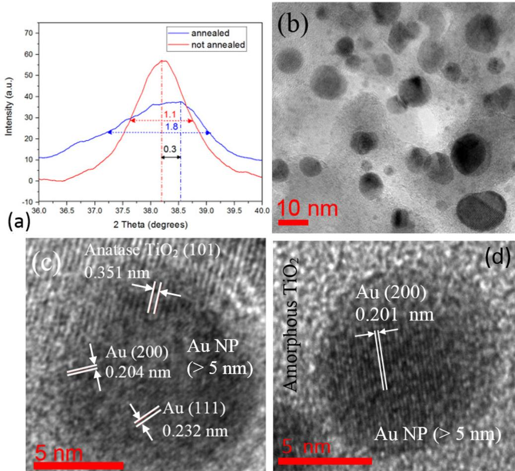
**Figure 4.** (a) XRD peak of the Au (111) in the Au-TiO<sub>2</sub> in pre- and post-annealing states; (b) Low magnification TEM image showing Au NPs in the annealed A-PLATEN; (c) and (d) HRTEM lattice fringe images of the Au NPs in annealed and un-annealed A-PLATENS respectively.
