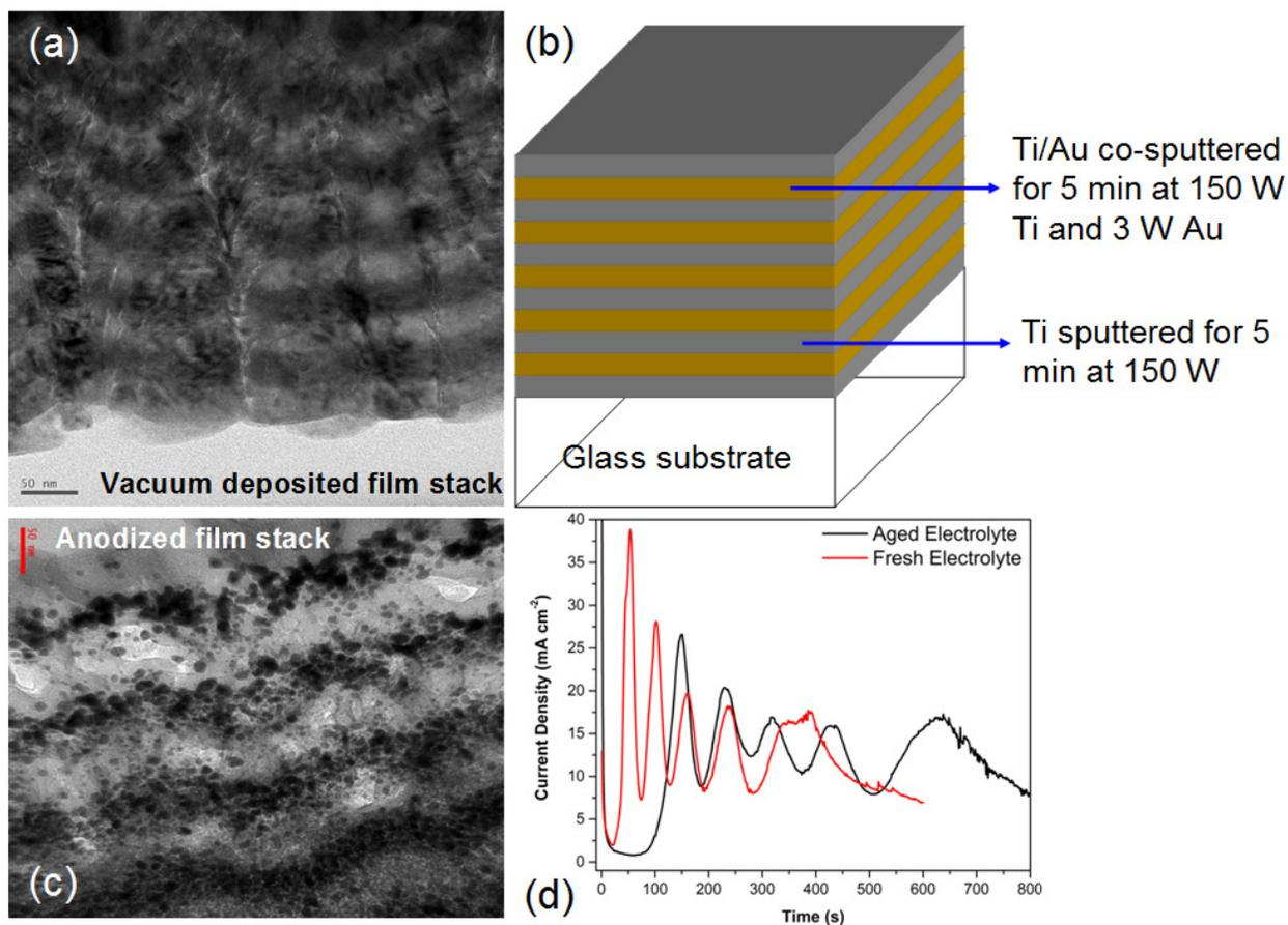
**Figure 1.** (a), (b) TEM cross-sectional image and schematic illustration of the thin film stack formed by sputtering alternate layers of Ti and Au-Ti on a glass substrate; (c) TEM image following anodization of the thin film stack showing bands of gold nanoparticles concentrated in regions corresponding to the Au-Ti layers
