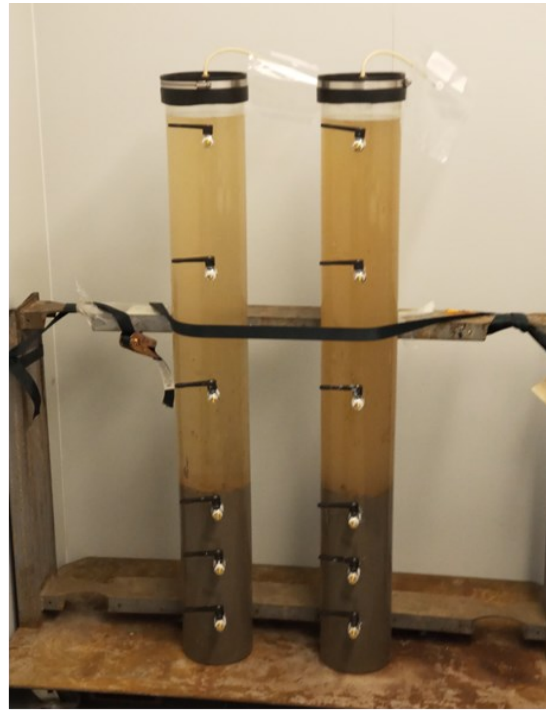
Figure 3.1: Laboratory experimental set up showing the column dimension and arrangement of sampling ports
