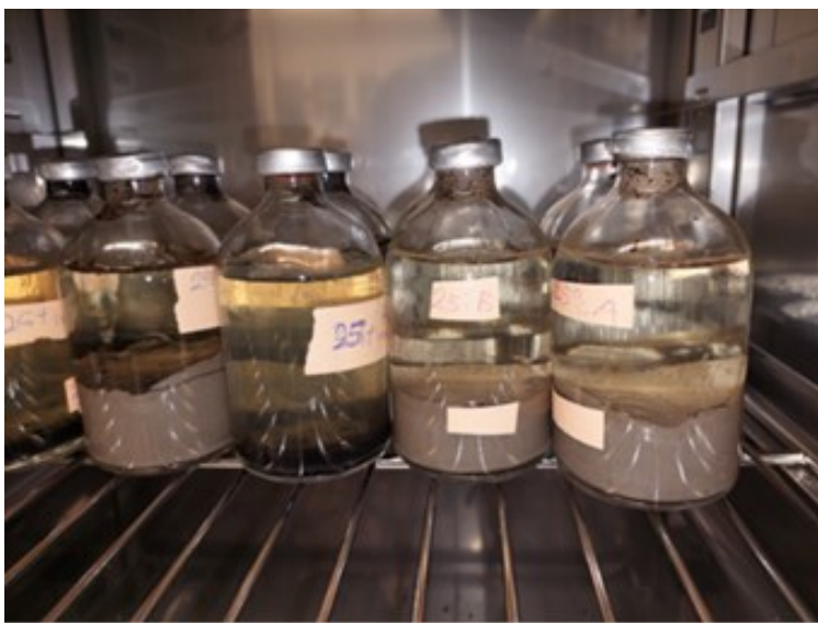
Figure 2.4: Serum bottle experiment showing tailings and capping water incubated at 25°C
