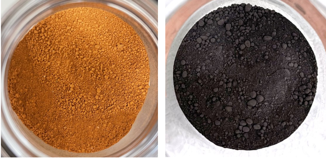
Figure 2. Images of raw bauxite residue (left) and calcined bauxite residue (CBR) (right)
