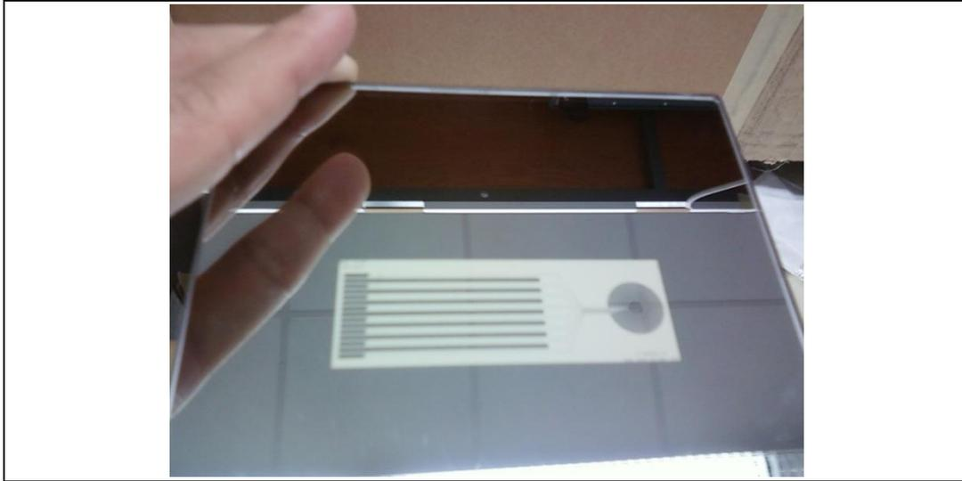
Fig.5.6. Fabricated annular array mask.
