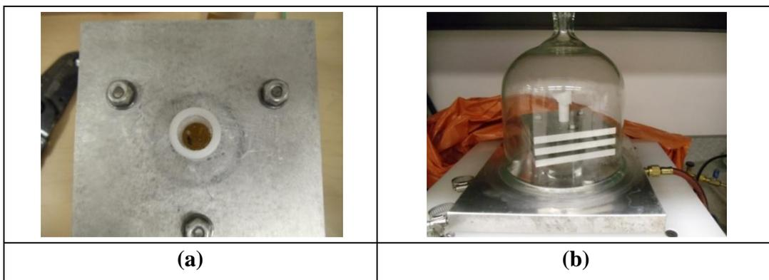
Fig.5.18. (a) Pouring out-gassed epoxy into the Teflon tube; (b) Out-gassing epoxy again.
