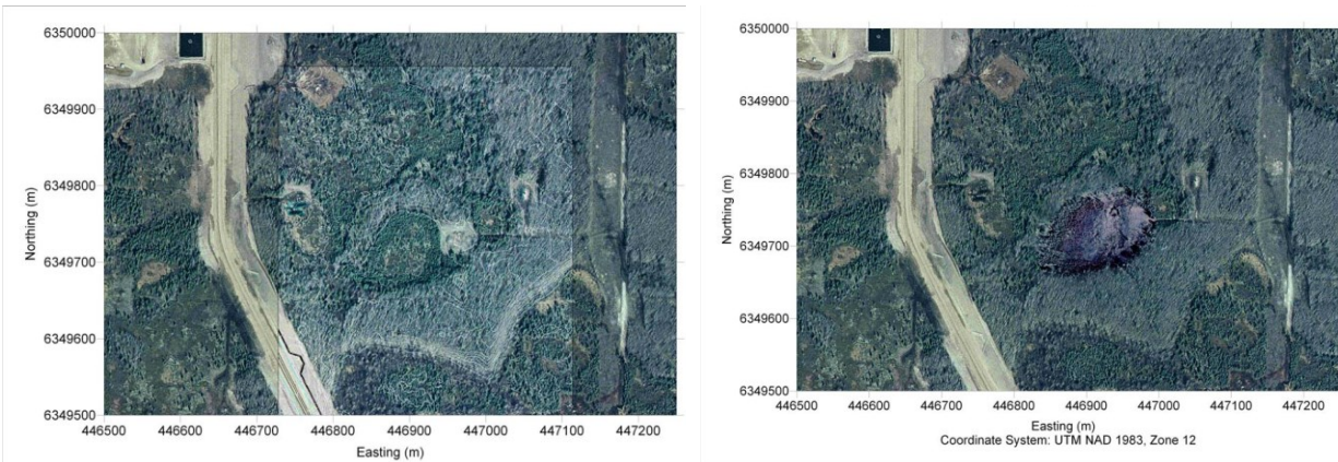
Figure 1-2 Aerial photography of the steam release area before and after the steam release (Total E&P Canada, 2007)
