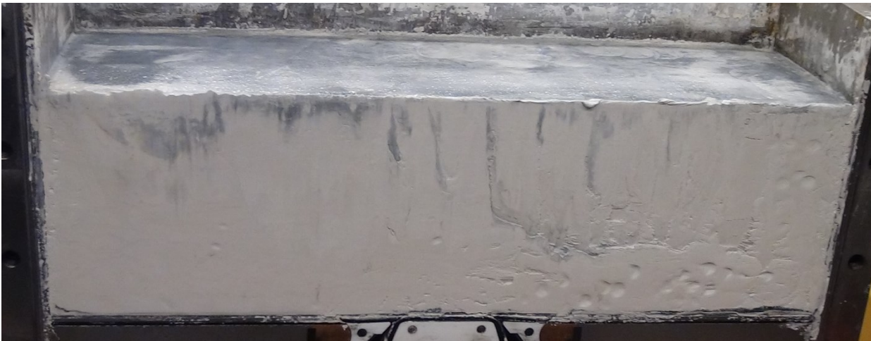
Figure 3-17 The front surface of the model polluted by the soil-water mixture
