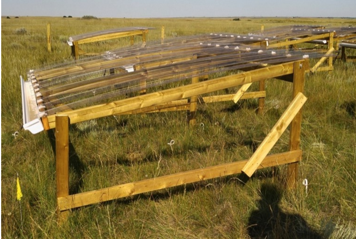
Figure 2.1 Rainout shelter to reduce rainfall (by 45%) for simulating drought conditions in the field.
