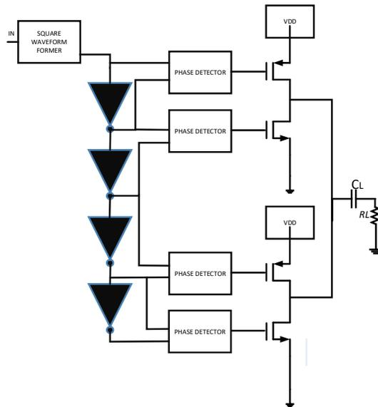
Fig. 20. Gaussian pulse generator [17]
