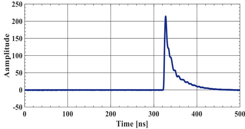
Fig.27 Marx Avalanche transistors output
