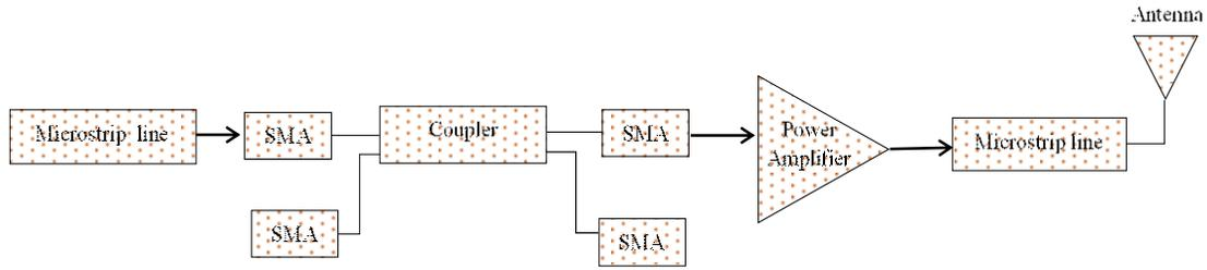
Fig.1 Gaussian pulse transmitter
