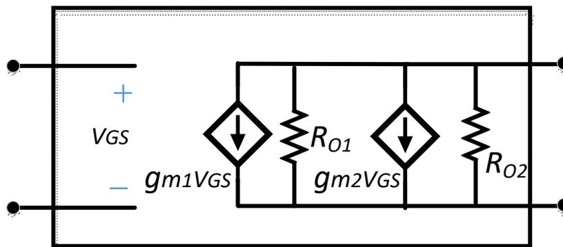
Fig. 40. Inverter two-port network model
