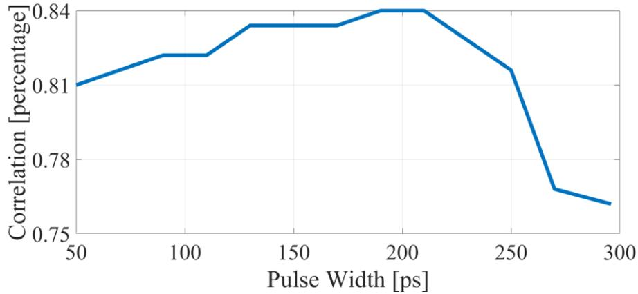
Fig. 11. correlation of ideal and real configurations as a function of pulse width
