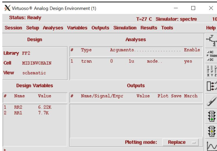
Fig.37 transient simulation setup
