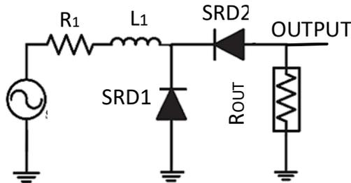
Fig. 16. Gaussian pulse generator by using SRD diodes [10]
