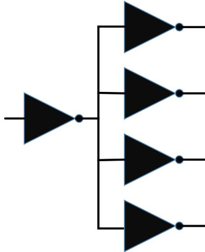
Fig. 41. An inverter connected to multiple branch circuit
