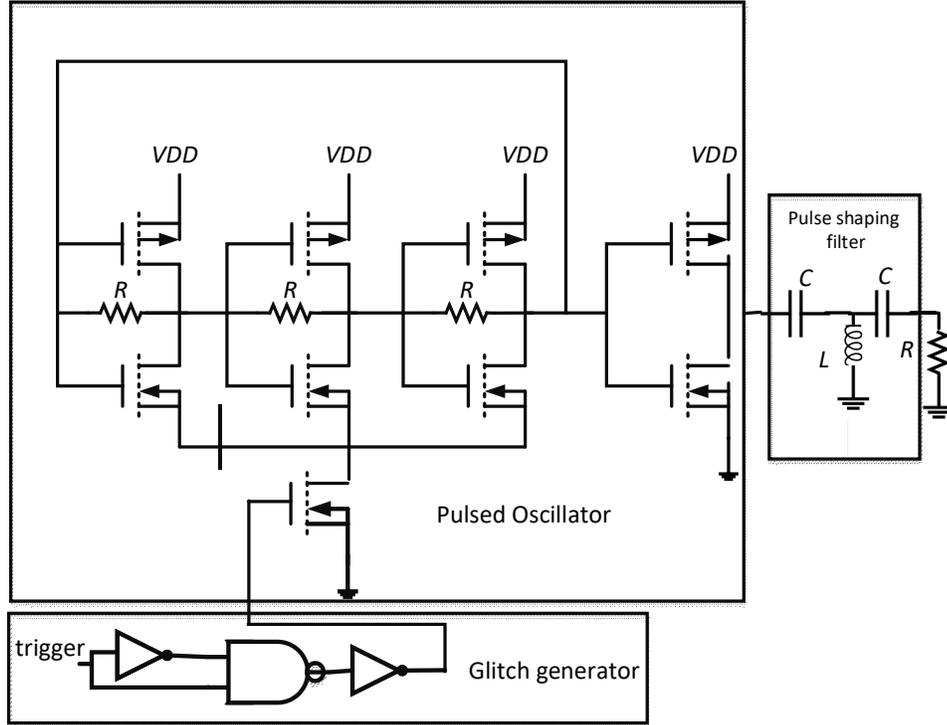
Fig. 18. Gaussian pulse generator by using an oscillator [32]
