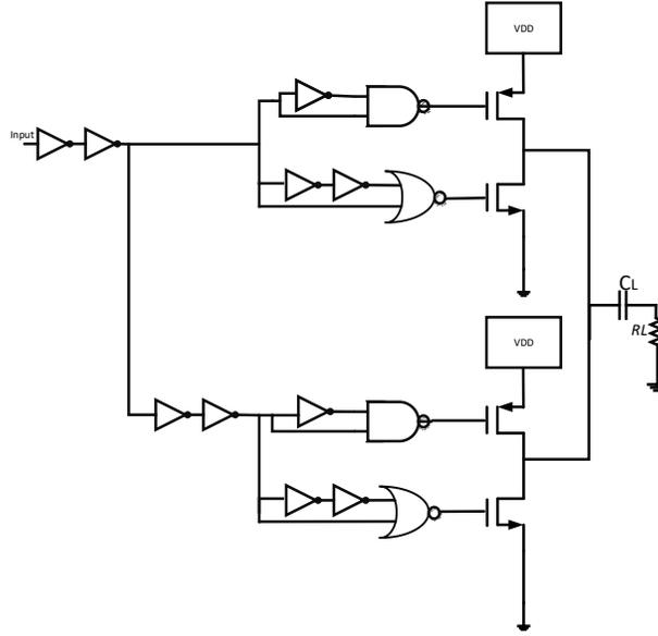
Fig. 19. the digital triangular pulse generator [33]
