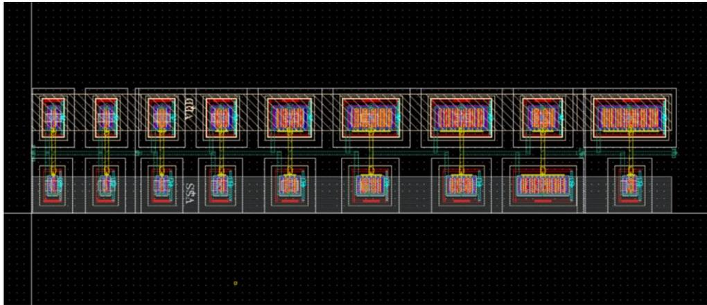
Fig. 54. a) First rising edge circuit Layout
