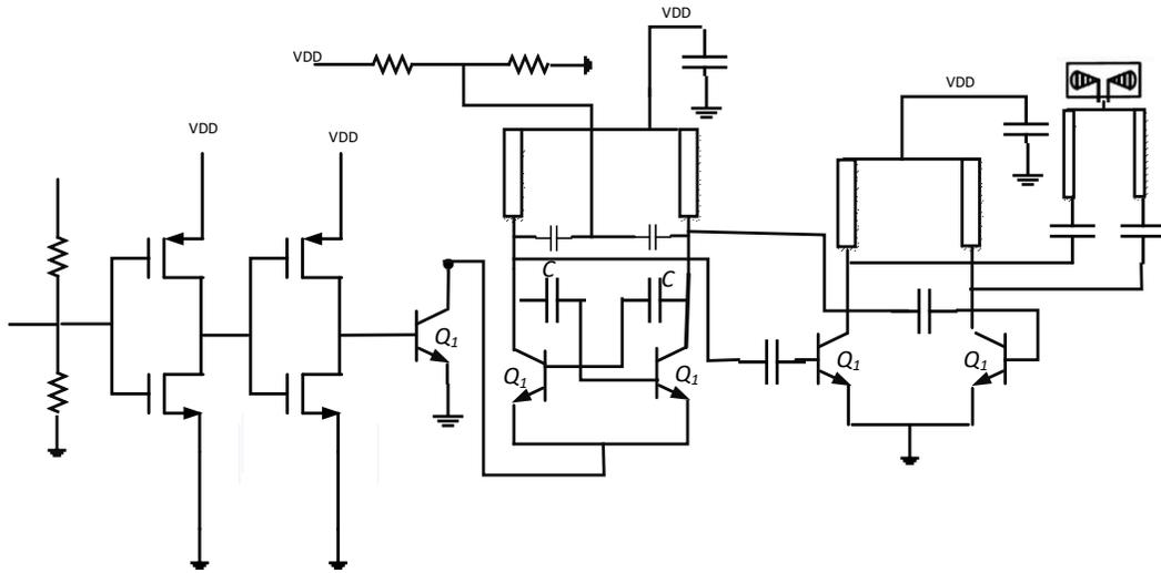
Fig.24 Gaussian pulse generator with Asymmetric VCO [35]
