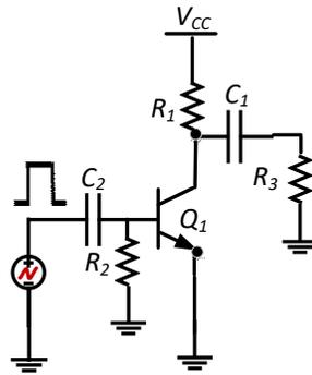
Fig. 17. Gaussian pulse generator by Avalanche transistor [9]
