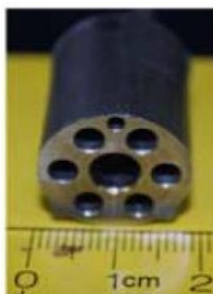
Figure 3.1 Six-shooter sample holder for in situ XAS data collection. The total diameter of the six shooter is 18 mm, and the diameter of each hole for the sample is 4 mm. The small hole at the top connects to the thermocouple, and the larger central hole is used for beam alignment
