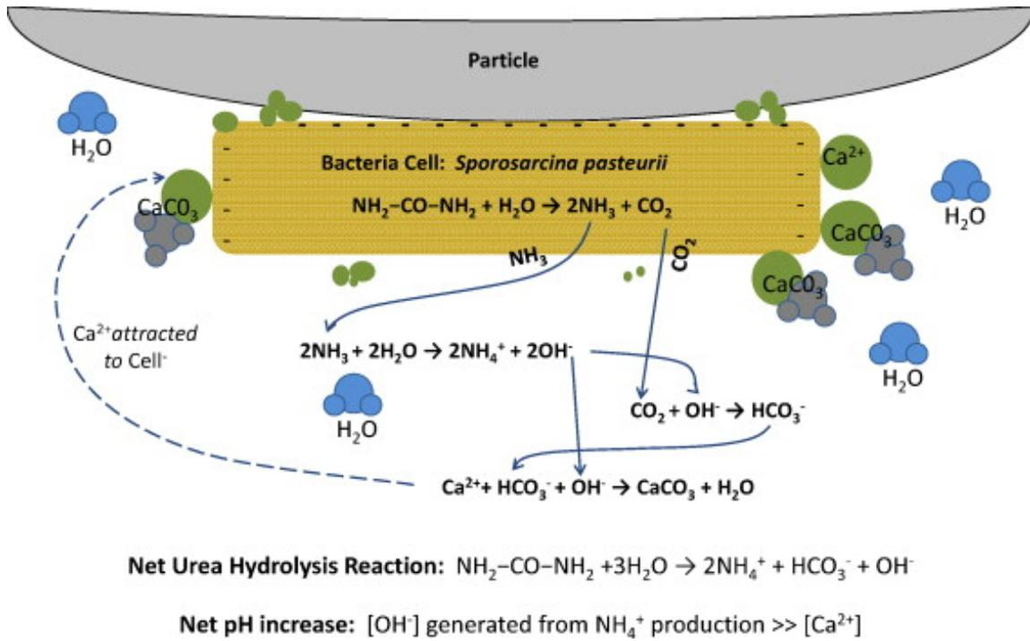
Figure 1.5: The mechanism involved in the MICP process is shown (DeJong et al., 2010).
