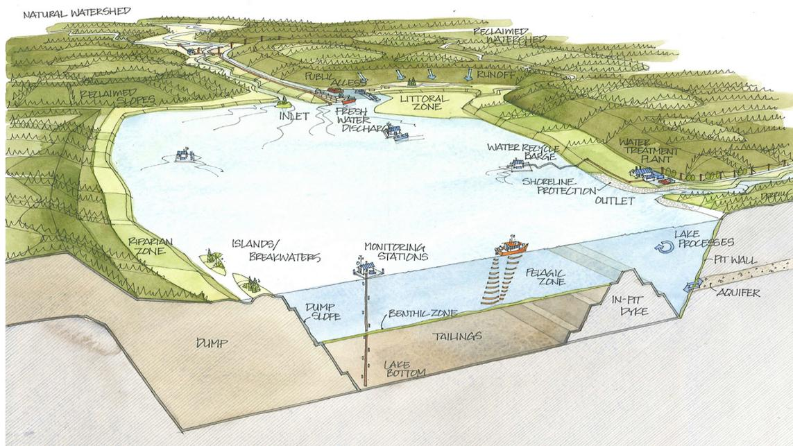
Figure 1.2: A conceptual model for an EPL with tailings: mature stage (Charette et al., 2010)
