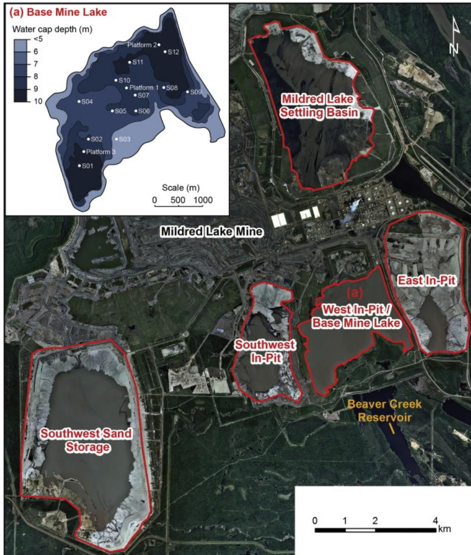
Figure 1.3: Oil sands tailings ponds and BML (WIP, the precursor tailings pond) are shown in the satellite image. Inset (a) shows a detailed image of the BML monitoring stations for the lakes monitoring program and water cap depth profile in 2016 (Dompierre and Barbour, 2016).
