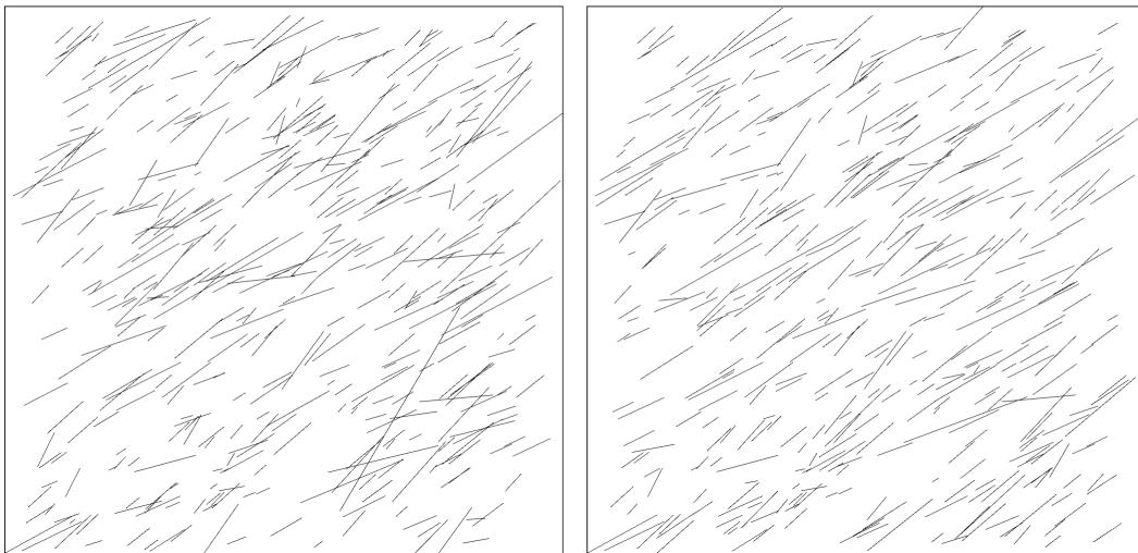
Figure 5.24: On the left: An initial DFN generated to represent the lineaments on the map of lineaments. On the right: The optimized DFN after 3400 iterations (visiting each of the 850 lineaments 4 times). 1 cm on the figure represents 8.2 km.
