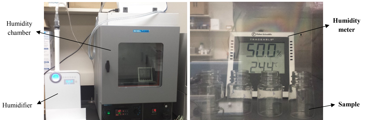
Figure 4-14. Capillary condensation experiments set up.
