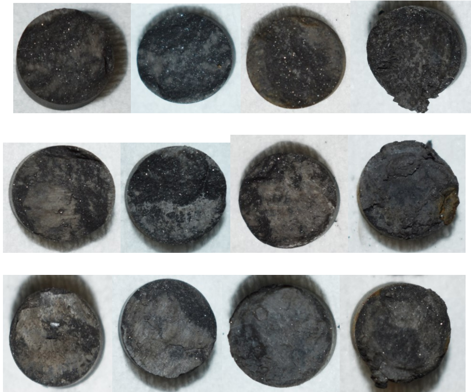
Figure 4-115. Sheared perpendicular samples in different water saturations. Top, middle and bottom images are related to 5MPa, 25MPa and 50MPa normal stress. In each normal stress from left to right the images are related to the water saturations of 7.8%, 31.3%, 51.9% and 81.8%.
