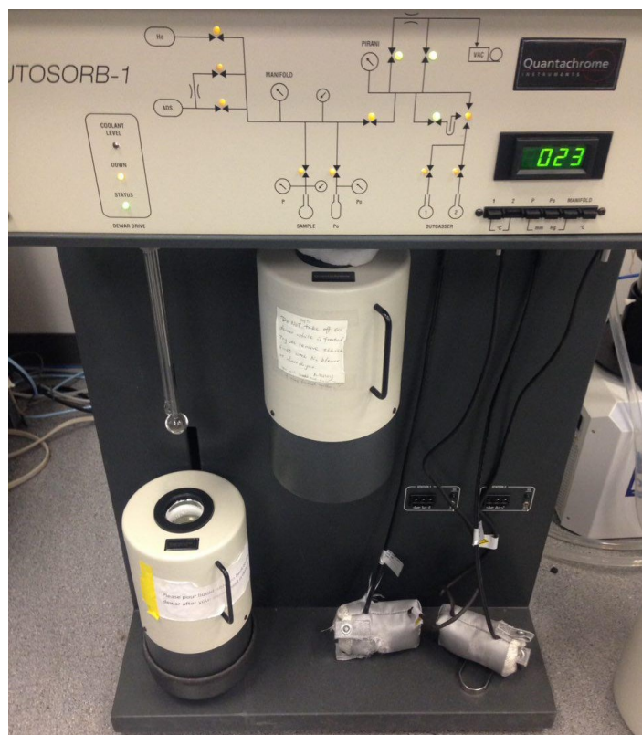
Figure 4-8. Autosorb Quantachrome 1MP device used for nitrogen adsorption–desorption Isotherms tests.
