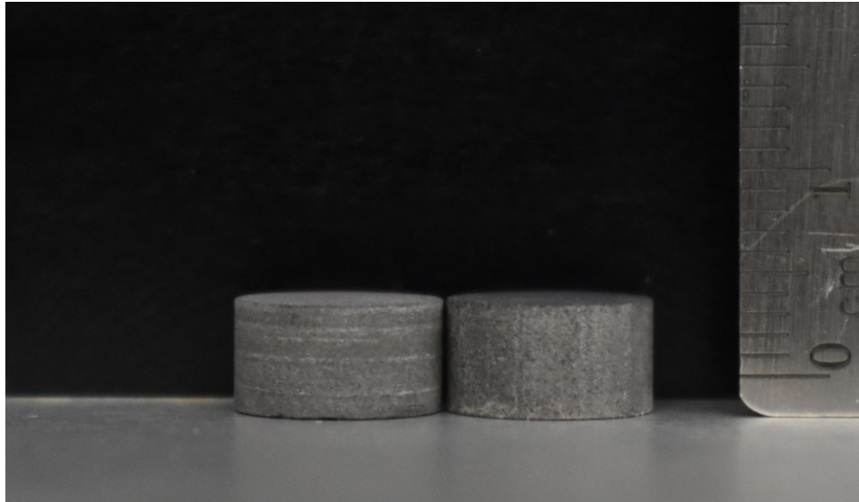
Figure 4-6. Preparing the samples of both parallel (right sample) and perpendicular (left sample) to the beds for direct shear tests.
