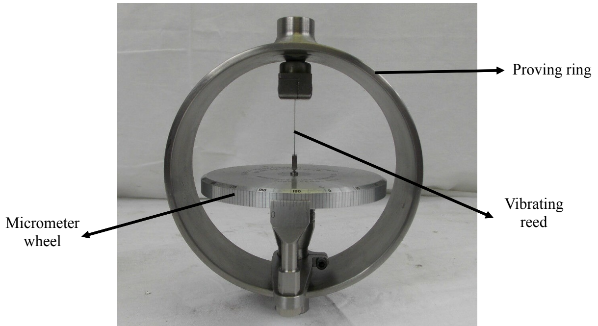
Figure 5-3. Proving ring applied for load cell calibration.
