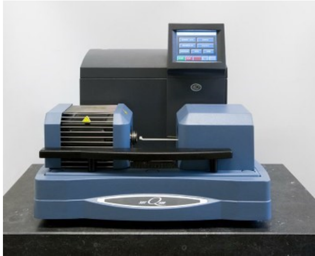
Figure 4-12. SDT Q600 used for Thermo-Gravimetric Analysis (TGA).
