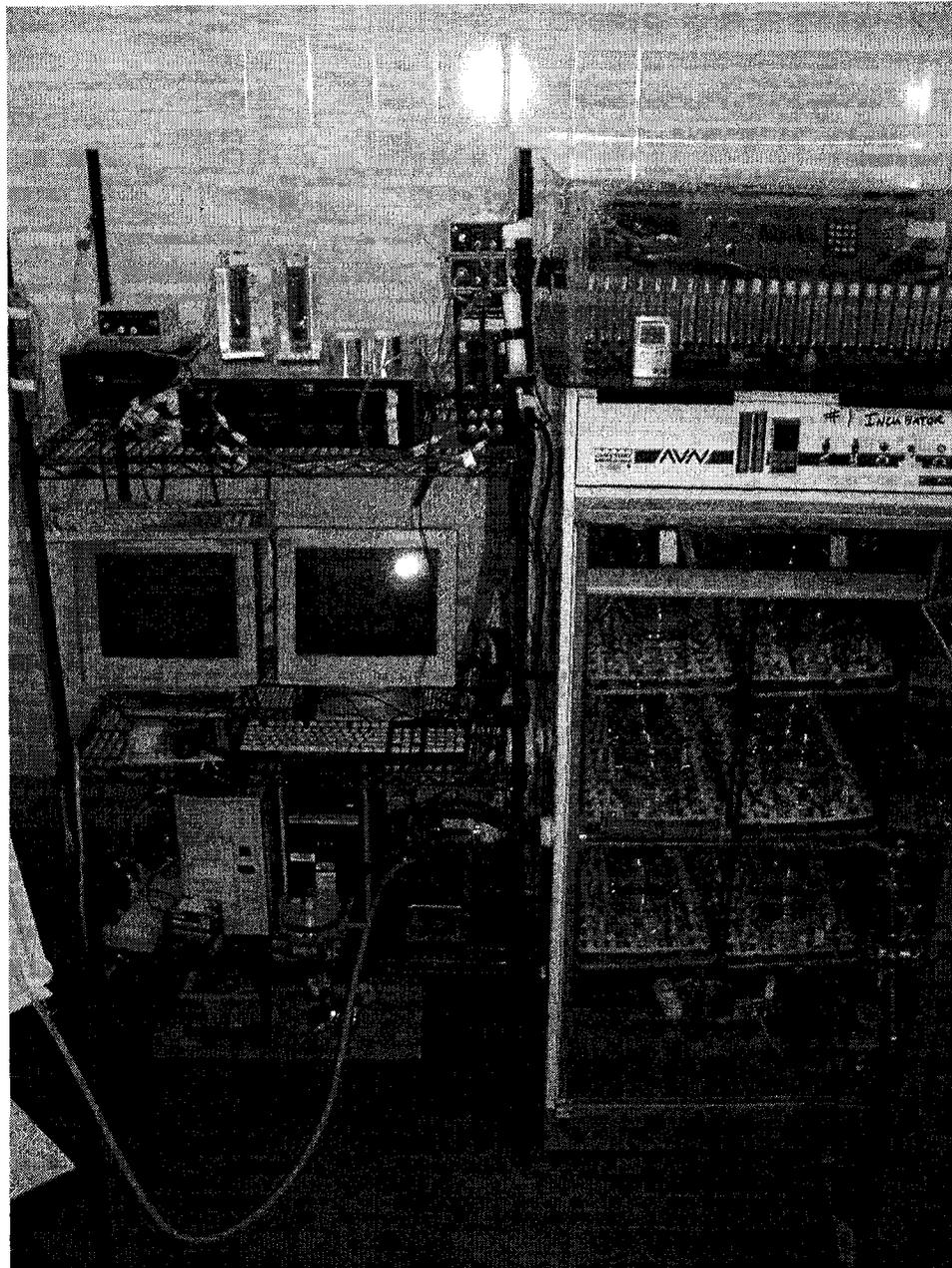
Figure 3: Egg metabolism equipment showing the incubator, metabolic chambers, CO<sub>2</sub>/H<sub>2</sub>O analyzer, differential O<sub>2</sub>, data recording computers and accessory parts
