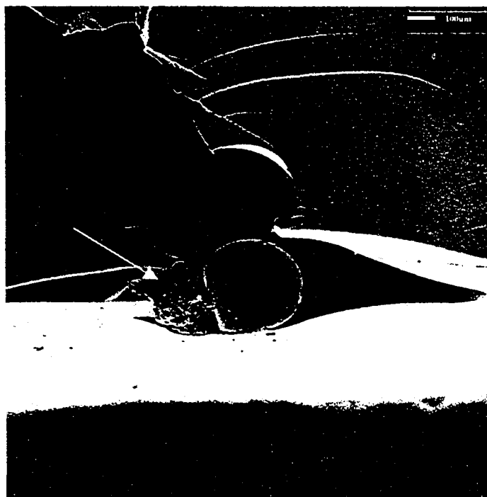
Figure 4.1. SEM micrograph of fracture surface of pure polyurethane after tensile test.
