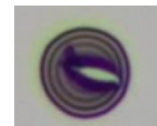
Figure 7. Optical image of a typical broken metal oxides based surface hollow nanolens.
