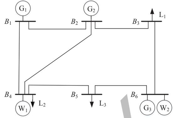
Fig. 1. Structure of 6-bus test system
