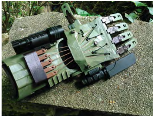
3D printed hand prosthetic with a tactical mounting system for military amputees
