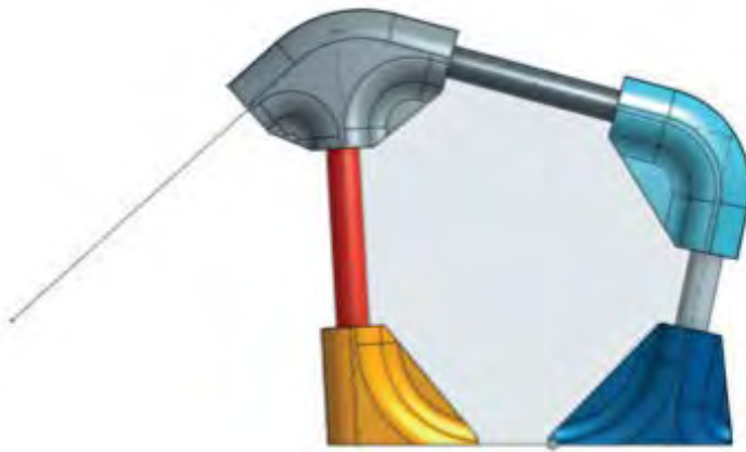
Figure 28 - OnShape is also parametric, in that the geometry updates with inputs
