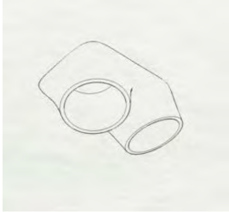
Figure 25: T-Splines Allow for more organic geometry
