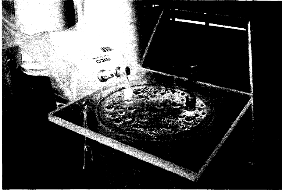
Figure 3.2 Top cover of dynamic column
