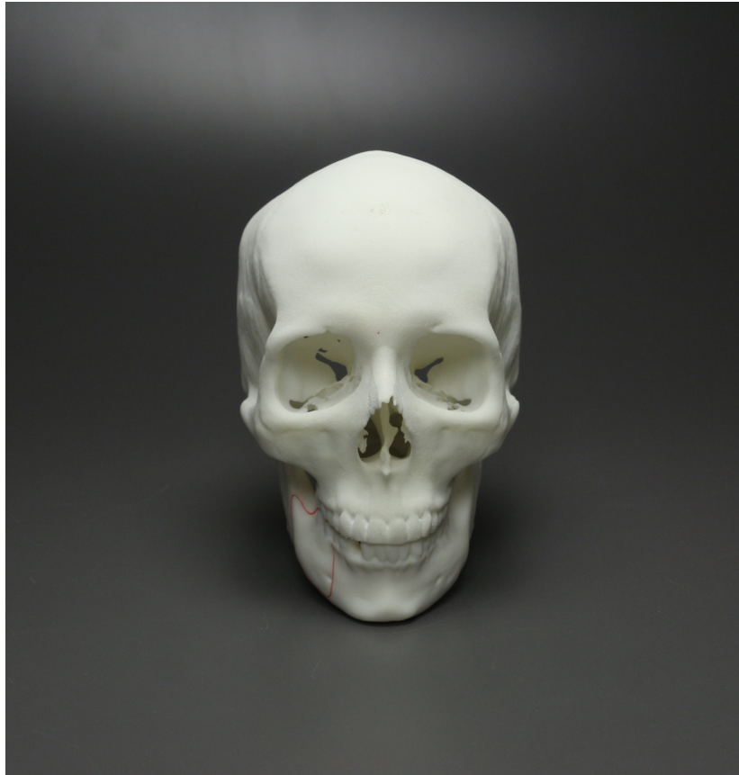
Fig 7. Additive-manufactured skull and mandible models
