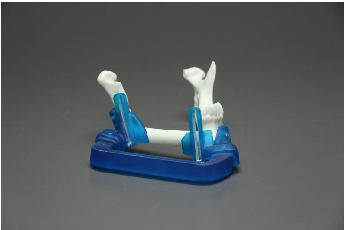
Fig 18. Mandible Fixation frame and cutting guides attached to a reconstructed mandible model.
