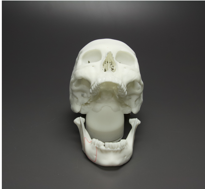
Fig 4. Additive-manufactured skull and mandible models.
