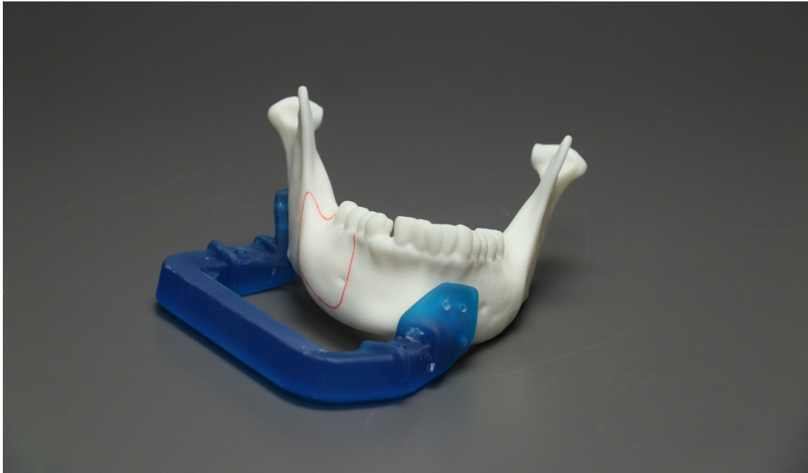
Fig 15. Mandible fixation frame attached to a complete mandible model.
