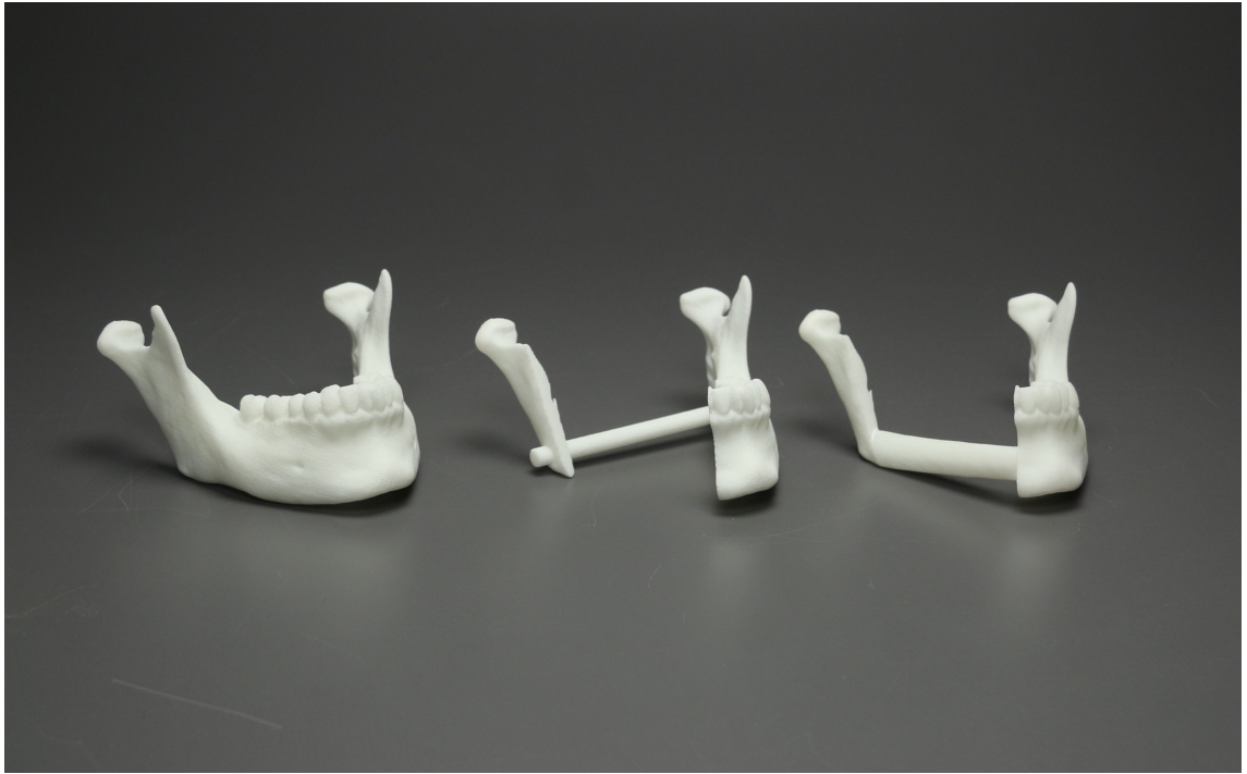
Fig21. Additive-manufactured reference models; complete, resected and reconstructed mandibles.
