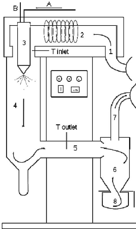
**Figure 1-8 Structure of a laboratory-scale spray dryer**
