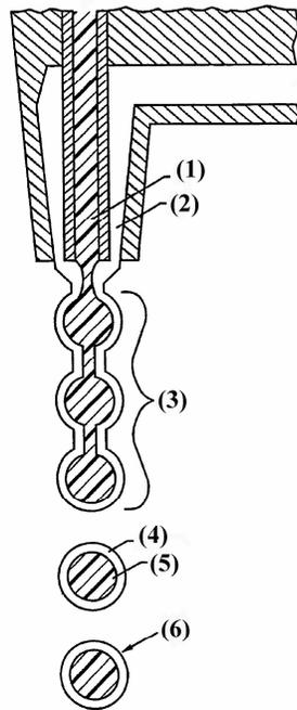
**Figure 1-9 Sectional view of an extrusion nozzle forming a microcapsule**
