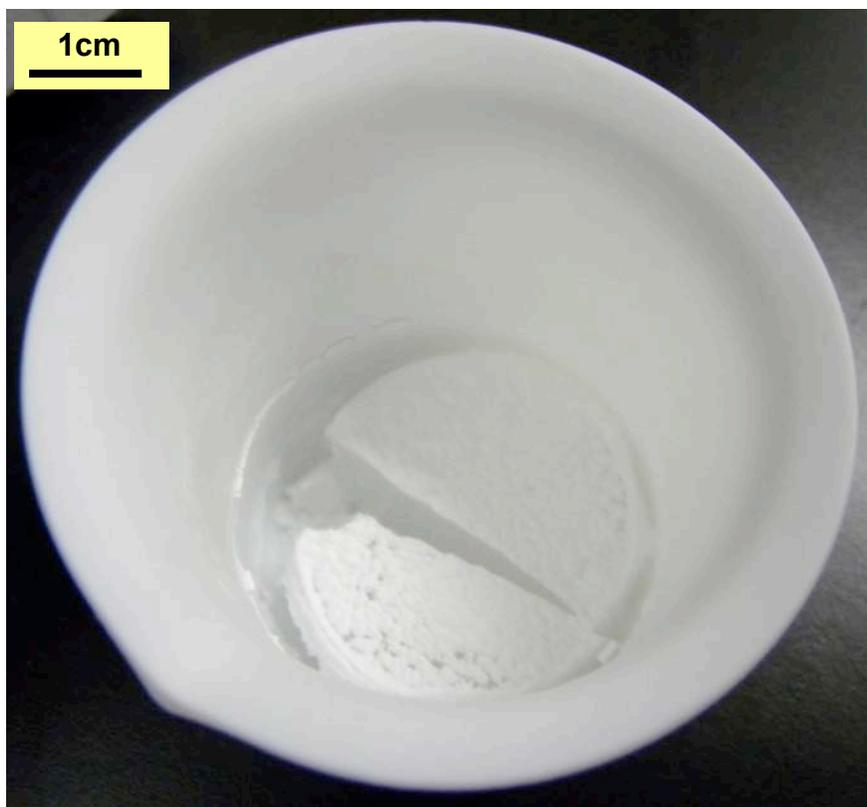
Figure 3-2 45S5 dried gel which formed after keeping sol for 1 day at 120°C temperature.
