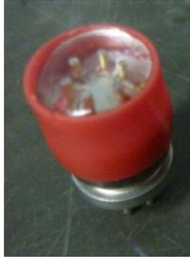
**Figure 4.6:** Feedthrough with crystal bond melted into the space between the pins. The red plastic is a cup to hold the crystal bond in place as it cools and solidifies.
