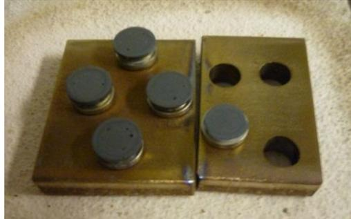
**Figure 3.16: Photograph of feedthroughs coated with Aremco Silicone Magnesia Low Melting Point Glass before firing.**
