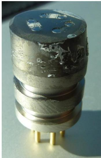
**Figure 4.4: Feedthrough with sample mount epoxy sacrificial layer at process step before electroplating and after photolithography.**
