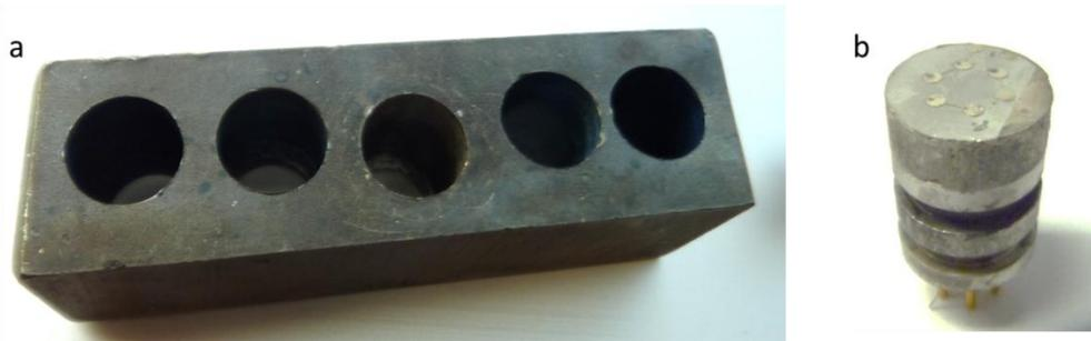
**Figure 4.7: a) Mild steel mold used to hold feedthroughs in place for molten solder to be poured over the pins. b) Feedthrough with a block of solid tin surrounding the pins with microfabricated devices on top.**
