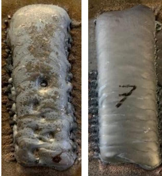
*Figure 12 View of the surface of samples fabricated with powder A (left) and powder B (right) using identical process parameters.*
