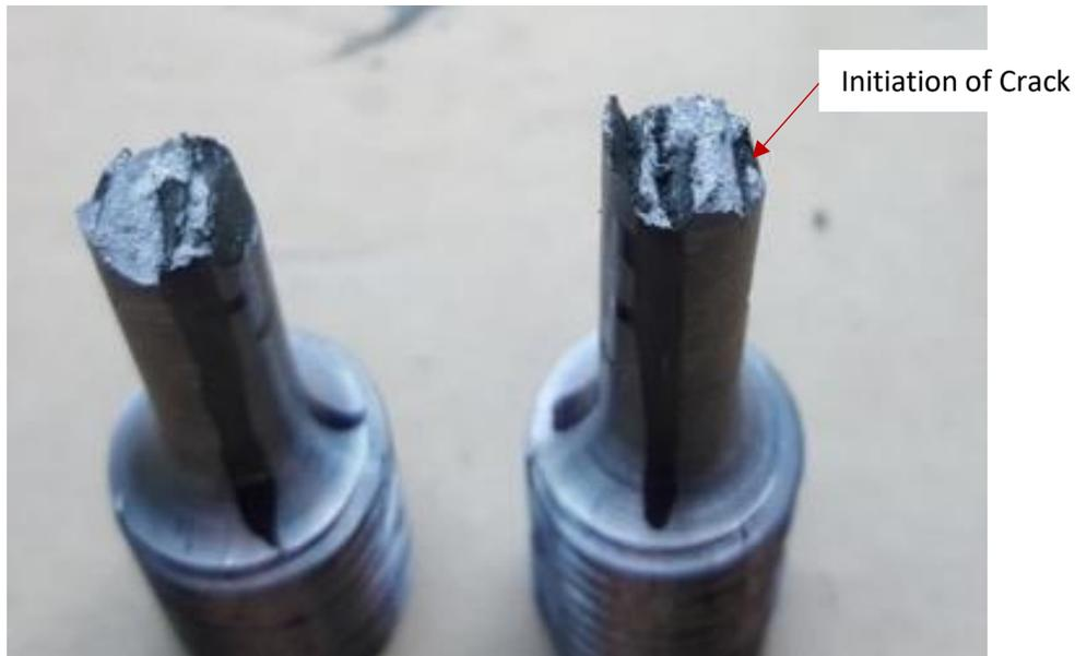
*Figure 8 Surface of tensile sample showing initiation of cracks along the oxide layers and the brittle fracture of the sample.*
