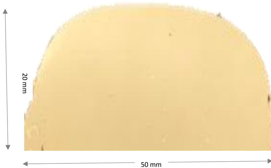
Figure 14 Cross section of deposit using powder B showing elimination of both the oxide layers (while using the shielding hood) and porosity.
