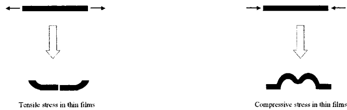
(a) Tensile stress causes a film to crack (b) Compressive stress causes a film to buckle
