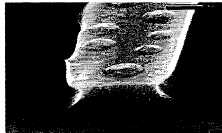
(e) End View of a bus waveguide.
