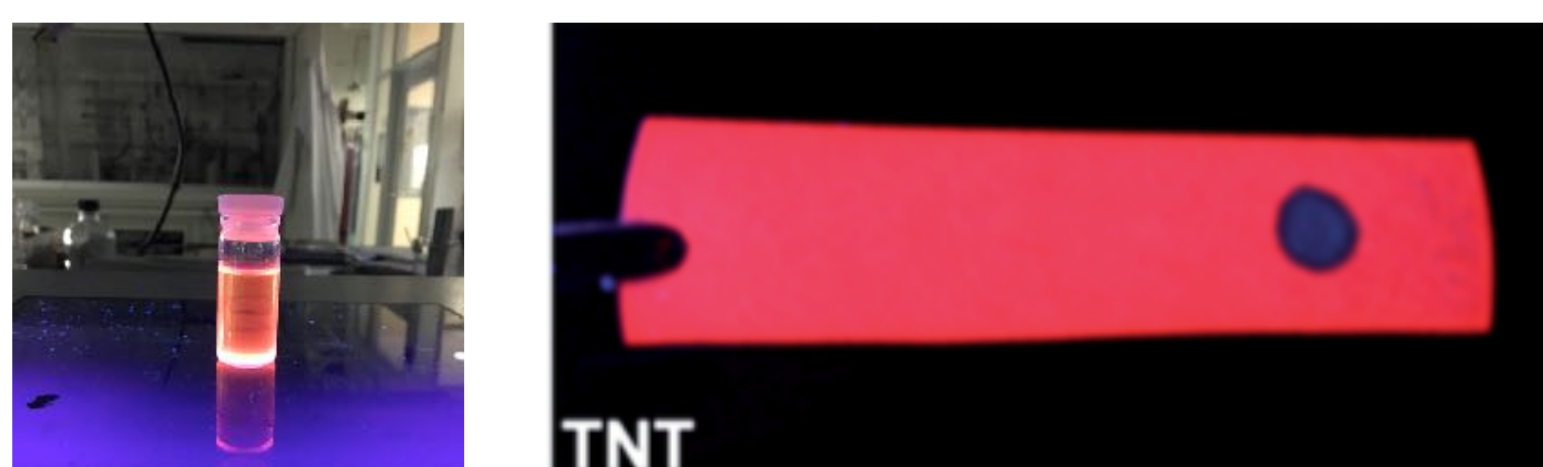
Figure 2: SiNC coated filter paper in the presence of nitroaromatic compound trinitrotoluene under UV light. Image from ref. 3.
