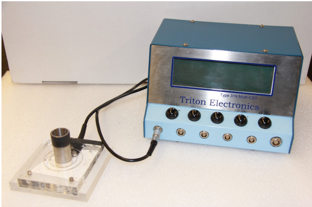
Figure 3-3 – Capillary suction testing schematic (left) and apparatus (right)
