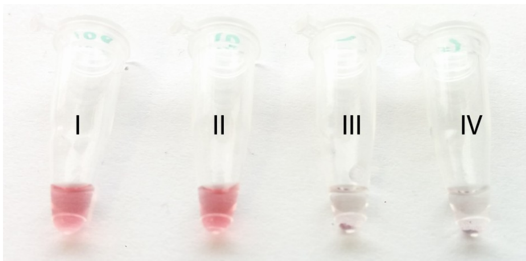
Figure 3.5. Target (OT 5 ) added to DNA-AuNP (150 fmol) and linker (OA 5 , 6 pmol). Target amounts used were i) 100 pmol, ii) 10 pmol, iii) 1 pmol, iv) no target.
