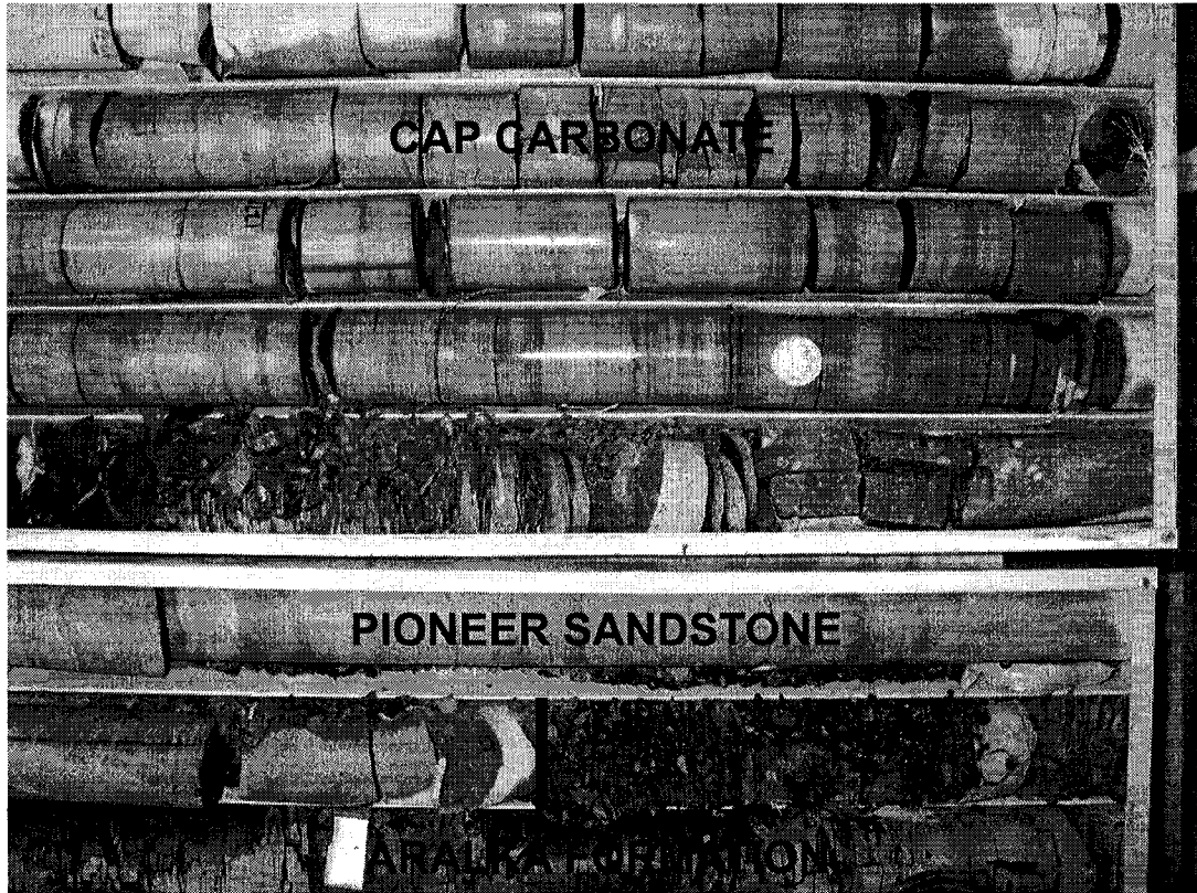
Plate 3.2: Aralka Formation and overlying Pioneer Sandstone and cap carbonate in drill hole Wallara-1. Vertical black bar represents the abrupt contact between the Aralka Formation and Pioneer Sandstone.
