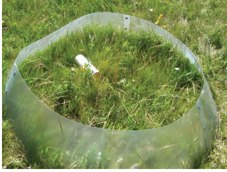
FIGURE 1: Close-up of an open-topped chamber (OTC) used to increase temperature within warmed grassland plots.
