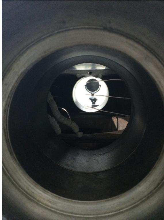
Figure 3.3: Temperature calibration image showing thermocouple positions.
