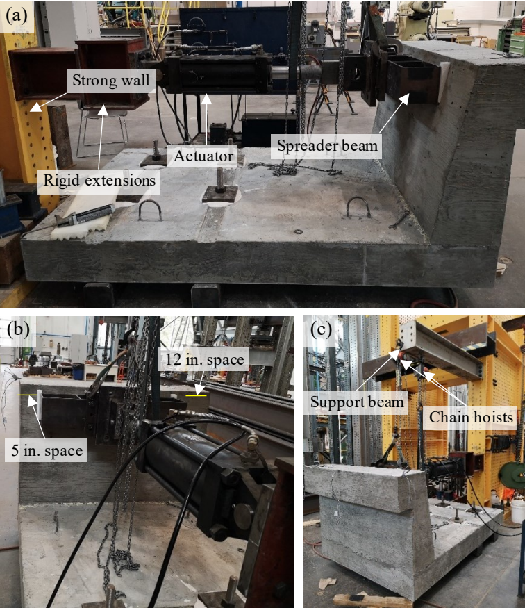
Figure C 2 Final test setup, (b) Spreader beam position along specimen's width, and (b) upper supporting structure composed of beam and chain hoists to maintain in a horizontal level the actuator.
