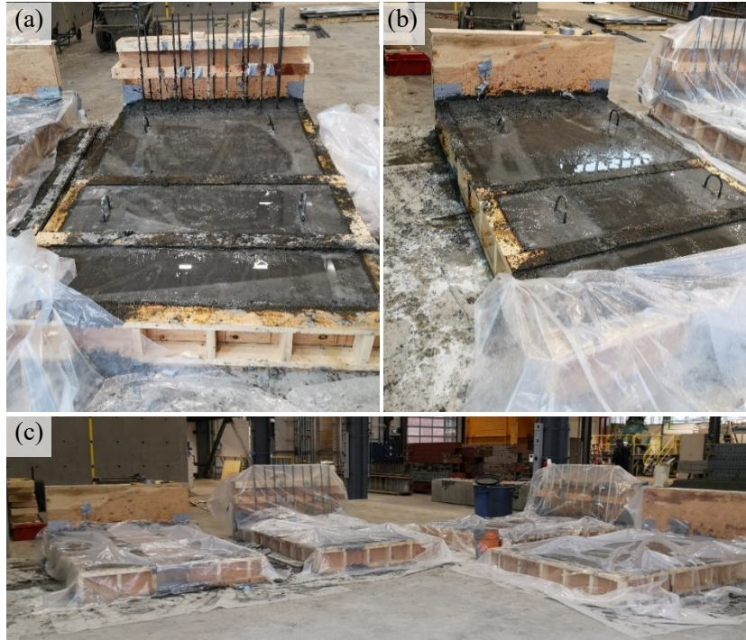
Figure A 7 (a and b) final product for SP-01 and SP-04 respectively, and (c) general photo of all specimens during curing.
