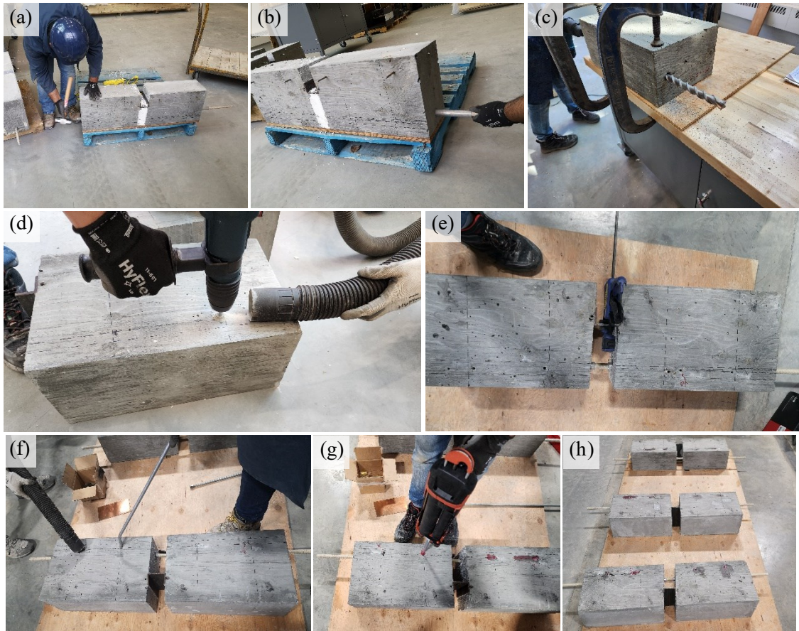
Figure B 2 (a) and (b) GFRP bar removal from hardened concrete, (c) hole wall roughening with rotary jack hammer, (d) lateral holes drilling, I beam segments positioning and levelling, (f) holes cleaned with pumped air, (g) epoxy resin injection into lateral cavities, and (h) specimens curing after epoxy injected.
