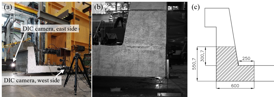
Figure 4.12 (a) DIC setup, (b) dotted area under analysis, and (c) DIC area dimensions.
