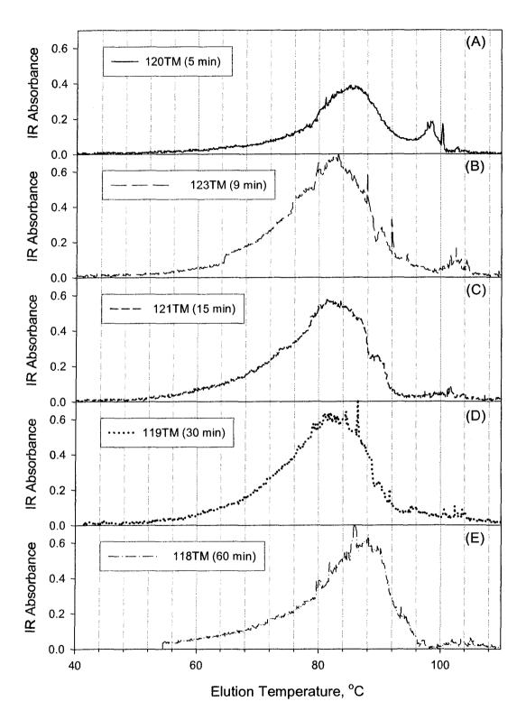
Figure 7.15: Effect of polymerization time on TREF profiles of copolymers showing elution curves for run of (A) 5, (B) 9, (C) 15, (D) 30, and (E) 60 minutes duration.
