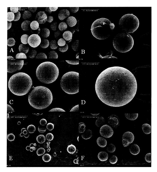
Figure 4.1: SEM images of supports of different sizes used for catalyst preparation – (A) 5  $\mu$ m PS/DVB-1; (B) 75-90  $\mu$ m HS-R6; (C) 125-150  $\mu$ m HS-R5; (D) 180-250  $\mu$ m HS-R3; (E) 250-300  $\mu$ m HS-R2; and (F) 600-850  $\mu$ m HS-R1
