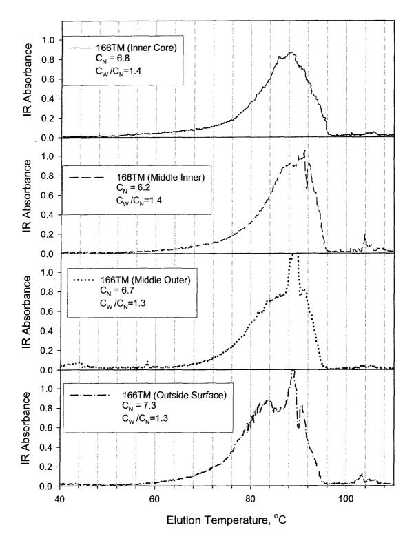
Figure 7.19: Variation of short chain branching with radial distance in a polymer particle.
