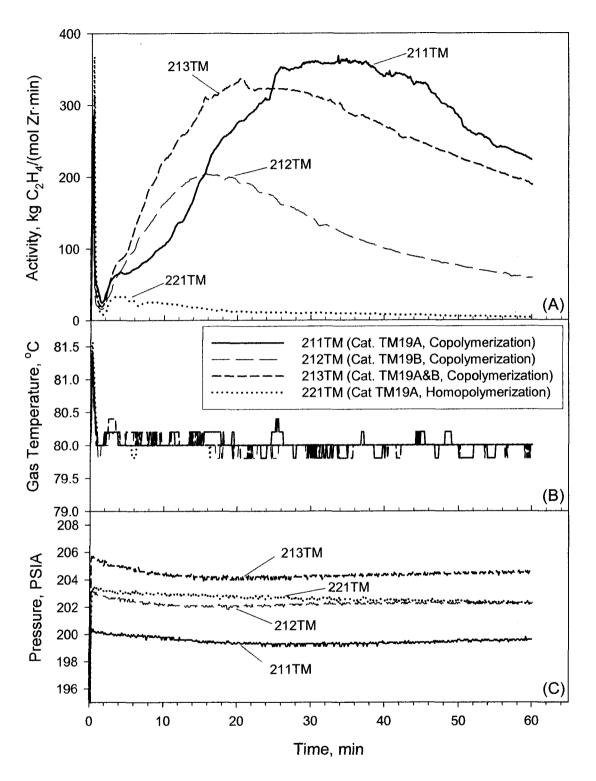
Figure 8.4: Effect of catalyst particle size on polymerization runs showing (A) activity profiles, (B) gas phase temperature profiles, and (C) pressure profiles.
