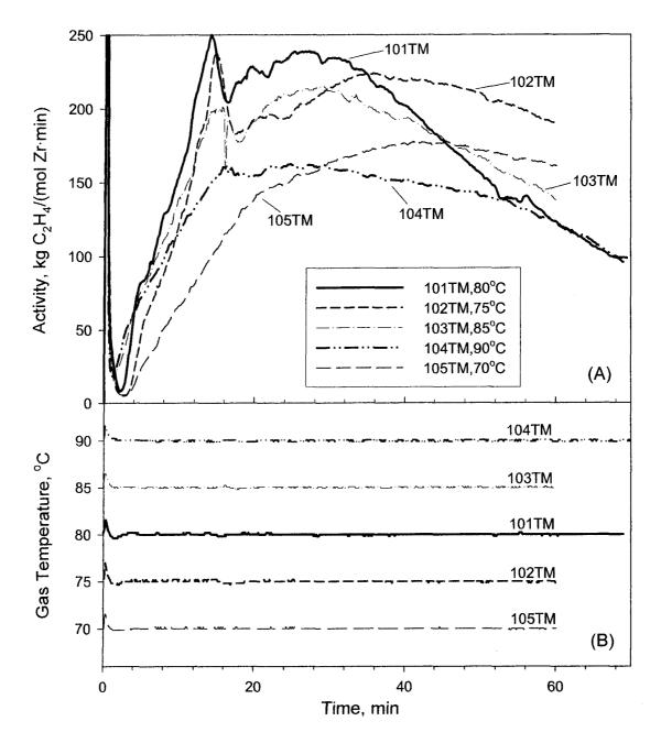
Figure 5.8: Effect of temperature on gas phase polymerization of ethylene and 1-hexene using Catalyst TM11 showing (A) activity profiles, and (B) temperature profiles.
