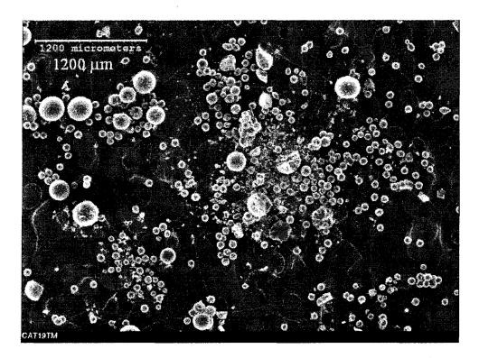
Figure 8.3: SEM image of Catalyst TM19 showing sizes of small (TM19A) and large (TM19B) particles.
