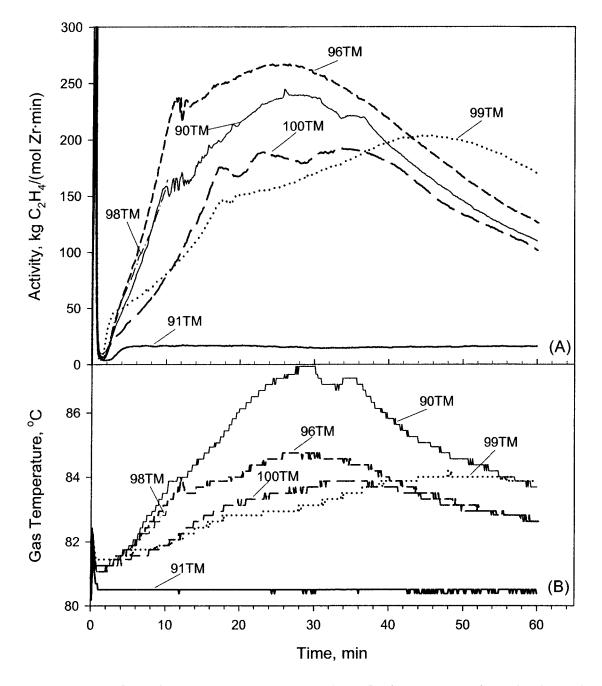
Figure 7.3: Effect of varying initial concentration of 1-hexene on polymerization using Catalyst TM11 showing (A) the activity profiles, and (B) the corresponding gas phase temperature profiles with circulation of coolant oil at 80°C to reactor.
