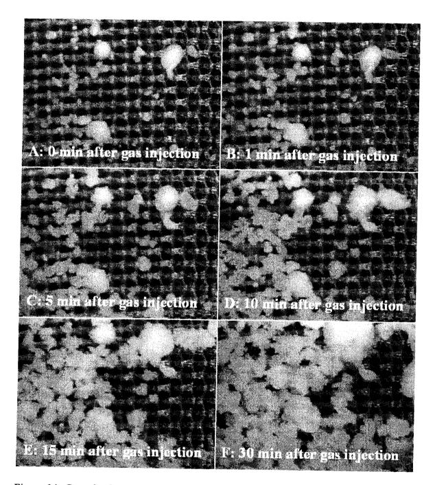
Figure 6.1: Growth of Catalyst TM15 (600–850  $\mu$ m support size range) particles and fragments on 250  $\mu$ m sieve during polymerization from (A) immediately after gas entry into micro-reactor to (F) 30 minutes later.
