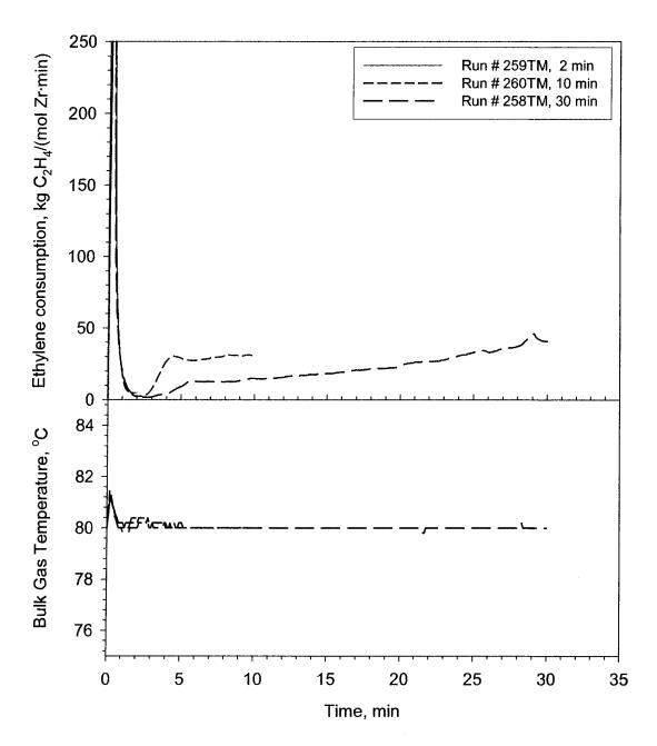
Figure 6.15: Activity and bulk gas temperature profiles of homopolymerization of ethylene using Catalyst TM22 at 80°C
