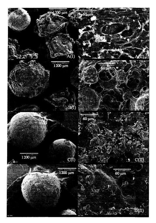
Figure 5.12: SEM images of polymer particles showing effect of gas phase polymerization temperature on outer morphologies at (A) 60°C (Run # 197TM), (B) 80°C (Run # 192TM), (C) 90°C (Run # 194TM), and (D) 100°C (Run # 196TM) using Catalyst TM17.
