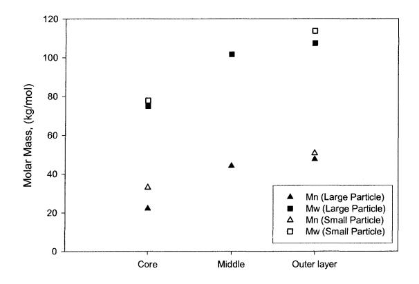
Figure 7.18: Variation of molar masses with radial distance in polymer particles (Large Particle  $\approx 8$  mm, and Small Particle  $\approx 4$  mm in diameter).
