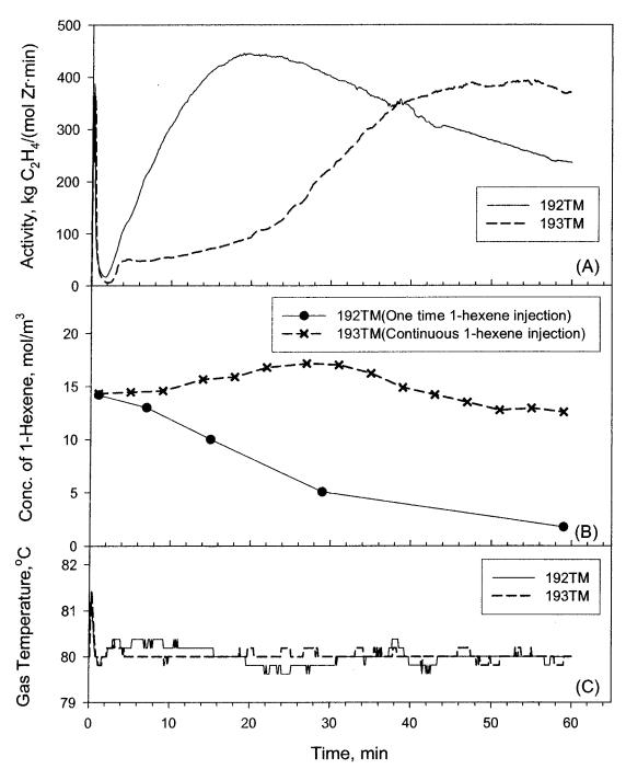
Figure 7.9: Effect of continuous injection of 1-hexene during polymerization at 1.4 MPa using Catalyst TM17 at 80°C showing (A) activity profiles, (B) concentration of 1-hexene, and (C) temperature profiles.
