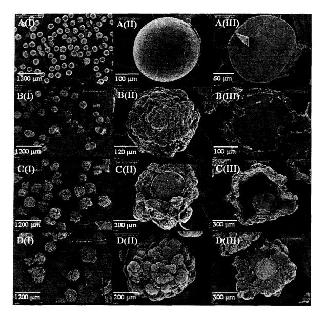
Figure 6.16: Homopolymerization with (A) Catalyst TM22 showing result of polymerization for (B) 2 minutes, (C) 10 minutes, and (D) 30 minutes at low, (I), and high, (II) and (III), magnifications for whole and cut particles.
