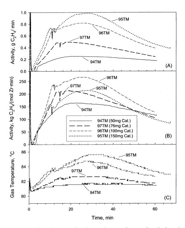
Figure 5.21: Effect of amount of catalyst used on gas phase copolymerization using Catalyst TM11 showing (A) activity profiles, (B) activity profiles per mole of zirconium, and (C) temperature profiles with coolant oil at 80°C circulating in reactor channels.
