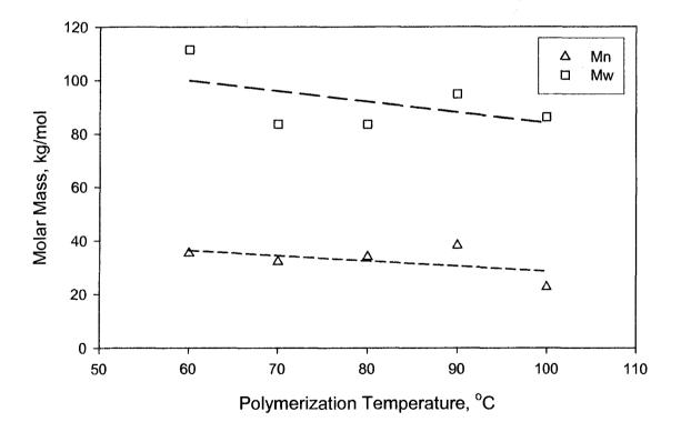
Figure 5.14: Effect of polymerization temperature on product polymer molar mass.
