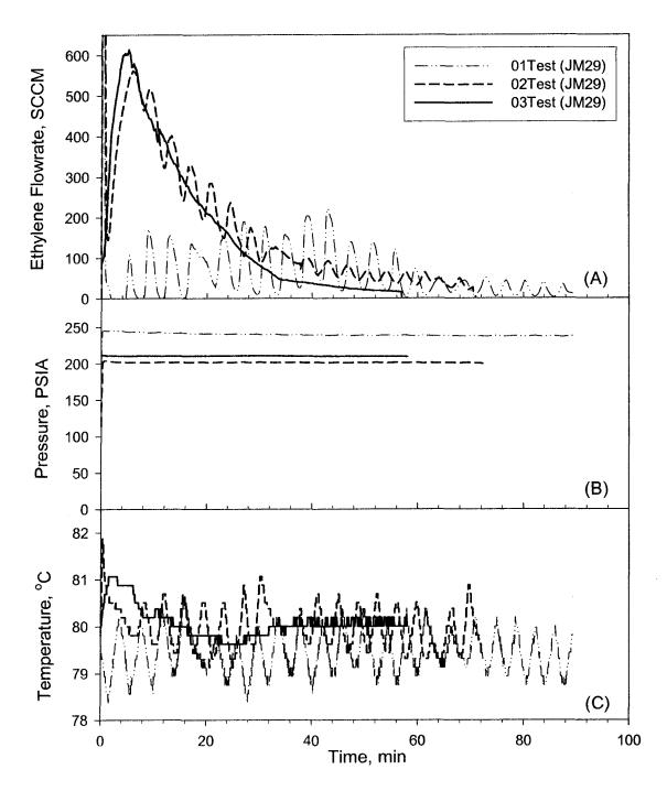
Figure 5.1: Effect of controller tuning on reaction profiles. Polymerization data from test runs using Catalyst JM29 showing (A) rate of ethylene flow into reactor, (B) reactor gas pressure, and (C) bulk gas temperature.
