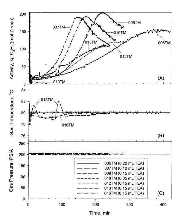
Figure 5.5: Effect of TEA (triethyl aluminum) on polymerization profiles (A) activity measured from flow rate of ethylene into reactor, (B) gas phase temperature, and (C) gas pressure
