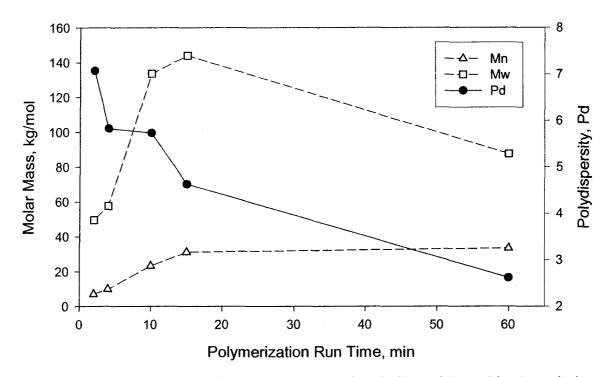
Figure 6.14: Development of molar masses and polydispersities with time during ethylene/1-hexene copolymerization at 70°C using Catalyst TM22.
