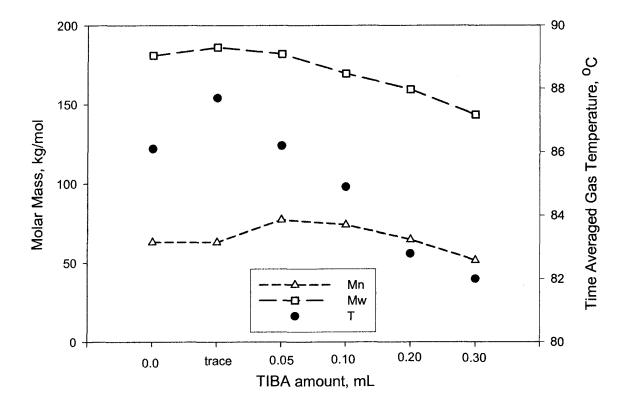
Figure 5.7: Effect of scavenger TIBA (tri-isobutyl aluminum) on PE molar masses, Mn and Mw, and time averaged gas phase temperature, T.
