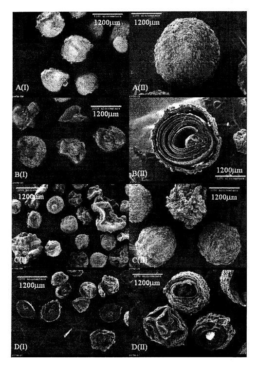
Figure 8.6: SEM images of Catalyst TM19 polymerized (I) small and (II) large particles, produced at 80°C, Run 214TM (A, B) and 70°C, Run 217TM (C, D) showing whole (A, C) and cut (B, D) particles.
