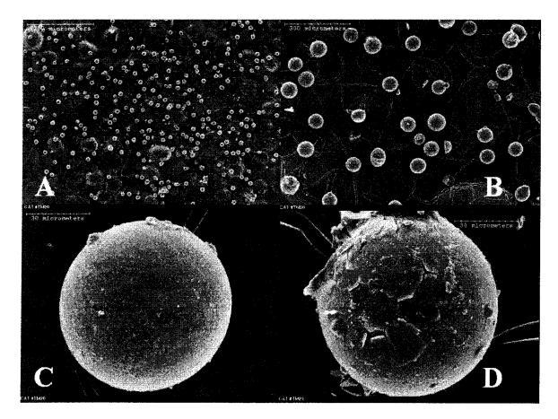
Figure 4.2: SEM images of catalyst TM20; (A) low magnification showing the uniform distribution of particle sizes; (B) higher magnification showing the catalyst particles having mainly uniform morphologies similar to support (HS-R6); (C) individual catalyst particle having relatively smooth surface; (D) individual particle having flaky surface.
