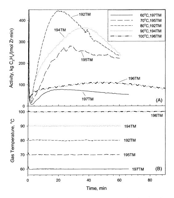
Figure 5.11: Effect of temperature on gas phase polymerization of ethylene and 1-hexene using Catalyst TM17 showing (A) activity profiles, and (B) temperature profiles.
