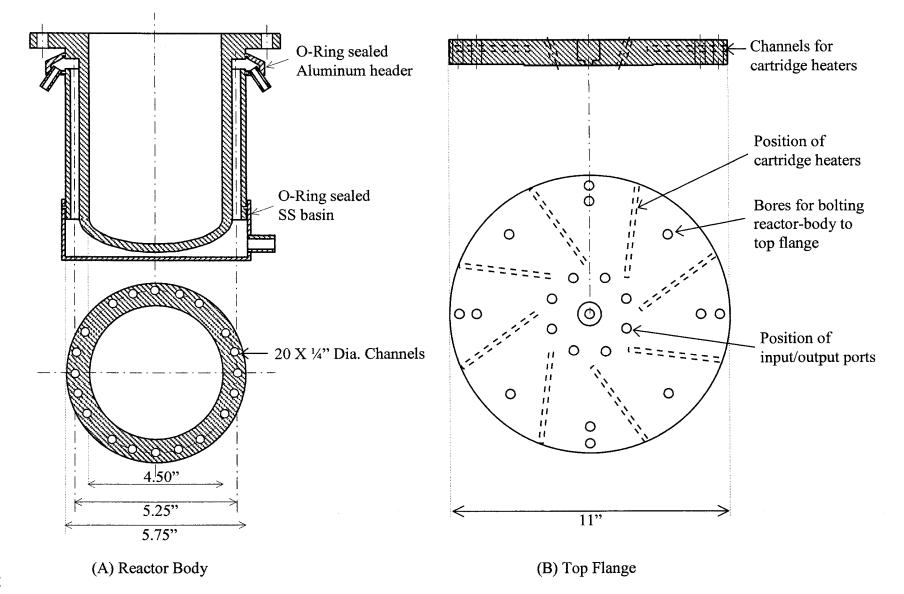
Figure 3.1 Schematic of Reactor Body and Top Flange Construction
