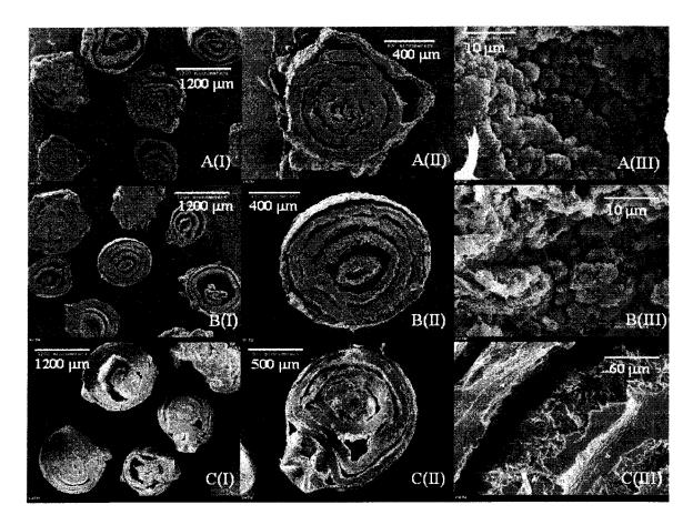
Figure 5.10: SEM images of polymer particles showing effect of gas phase polymerization temperature on inner morphologies at (A)  $70^{\circ}$ C (Run # 105TM), (B)  $80^{\circ}$ C (Run # 101TM), and (C)  $90^{\circ}$ C (Run # 104TM) using Catalyst TM11.
