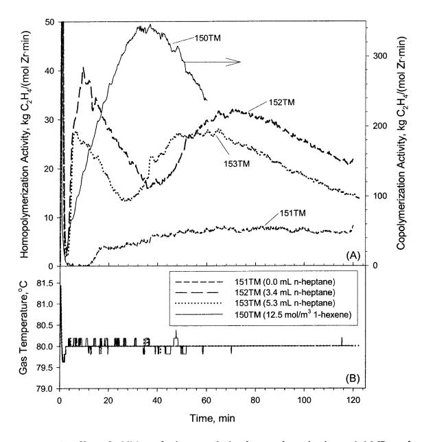
Figure 7.11: Effect of addition of *n*-heptane during homopolymerization at 1.4 MPa and 80°C using Catalyst TM15 showing (A) activity profiles, and (B) temperature profiles and compared to activity during copolymerization with 1-hexene (secondary Y-axis).
