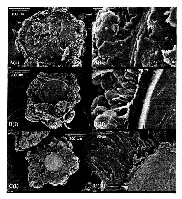
Figure 6.17: SEM of homopolymer particles showing radial growth of polymer outwards from catalyst core after (A) 2 minutes, (B) 10 minutes, and (C) 30 minutes of polymerization.
