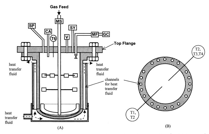
Figure 3.2. Schematic of Assembled Reactor: A) Radial Thermocouples not shown, B) Position of Radial Thermocouples (CA – catalyst injector; GC – gas chromatograph; MF – mass flow meter; MS – Magnedrive stirrer; SP – syringe pump; SY – syringe injection port;  $T_i$  – thermocouple *i* mounted as shown; V – vent)
