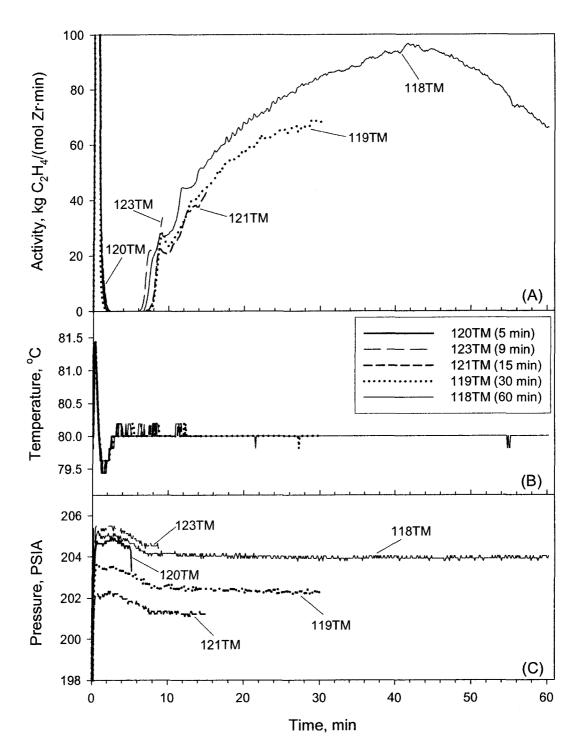
Figure 7.13: Catalyst TM12 catalyzed polymerization runs of various durations showing (A) activity profiles, (B) temperature profiles, and (C) pressure profiles.
