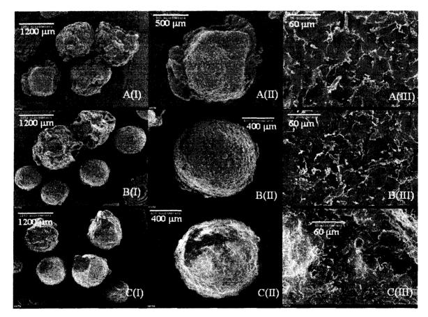
Figure 5.9: SEM images of polymer particles showing effect of gas phase polymerization temperature on outer morphologies at (A)  $70^{\circ}$ C (Run # 105TM), (B)  $80^{\circ}$ C (Run # 101TM), and (C)  $90^{\circ}$ C (Run # 104TM) using Catalyst TM11.
