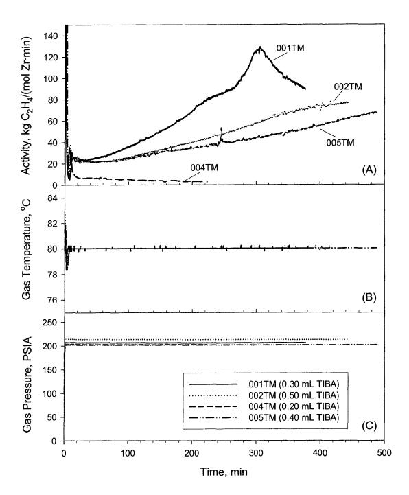
Figure 5.4: Effect of TIBA (tri-isobutyl aluminum) on polymerization profiles (A) activity measured from flow rate of ethylene into reactor, (B) gas phase temperature, and (C) gas pressure.
