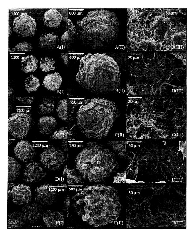
Figure 5.16: SEM images of polymer particles showing effect of gas phase pressure on outer morphologies at (A) 0.70 MPa (Run # 74TM), (B) 1.05 MPa (Run # 76TM), (C) 1.39 MPa (Run # 78TM), (D) 1.74 MPa (Run # 77TM), and (E) 2.06 MPa (Run # 75TM) produced by polymerization at 80°C using Catalyst TM10.
