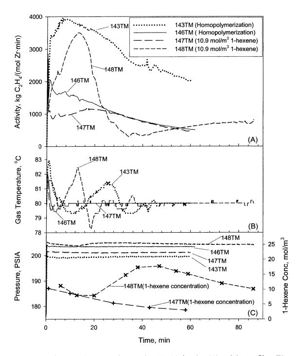
Figure 8.1: Polymerization runs using Catalyst TM14 showing (A) activity profiles, (B) gas phase temperature profiles, and (C) pressure profiles and concentration of 1-hexene.
