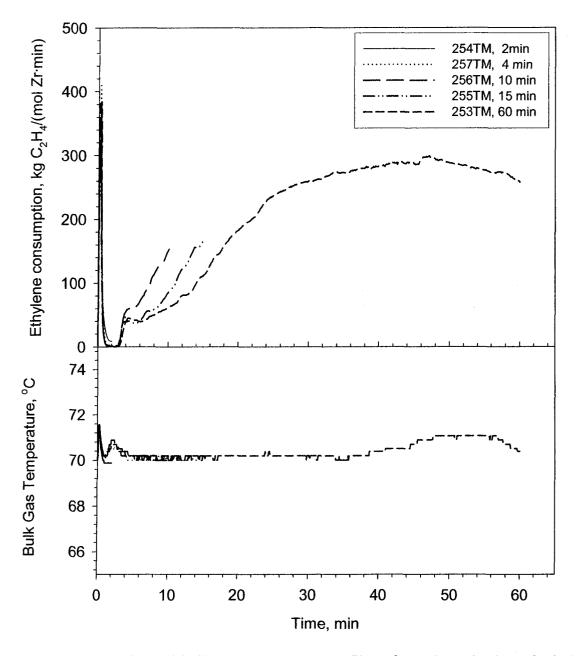
Figure 6.8: Activity and bulk gas temperature profiles of copolymerization of ethylene and 1-hexene with Catalyst TM22 at 70°C.
