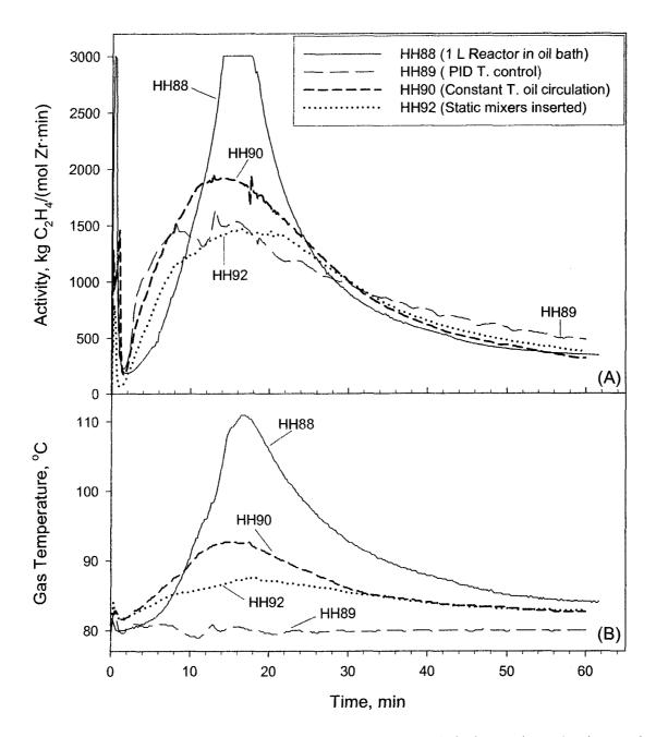
Figure 5.3: Comparison of gas phase temperature control during polymerization under various modes of operation showing (A) activity profiles, and (B) the corresponding temperature profiles.
