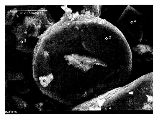
Figure 4.4 Fragmented TM19A particle for EDX probe analysis showing probe positions Table 4.2: Elemental analysis of probe positions showing normalized mass percentage
