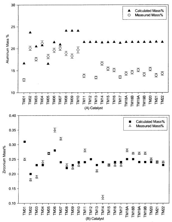
Figure 4.6: (A) Aluminum and (B) zirconium concentrations in catalysts, calculated from amounts of reagents used and measured using instrumental neutron activation analysis.
