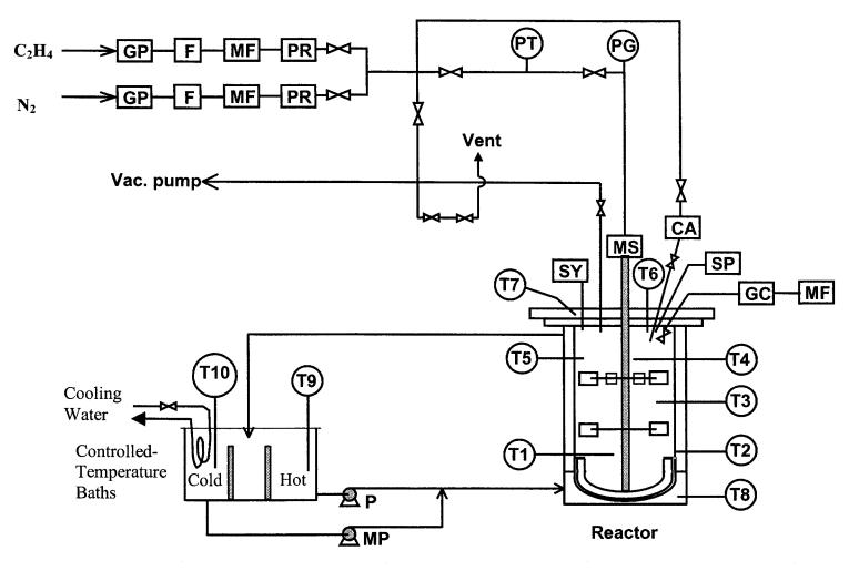
Figure 3.3. Schematic of Reactor System. (CA – catalyst injector; GC – gas chromatograph; GP – gas purifiers;  $F - filter 7 \mu m$ ; MF – mass flow meter; MP – metering pump; MS – Magnedrive stirrer; P – centrifugal pump; PG – pressure gauge; PR – pressure regulator; PT – pressure transducer; SP – syringe pump; SY – syringe injection port;  $T_i$  – thermocouple *i* mounted as in figure 2; V – vent)
