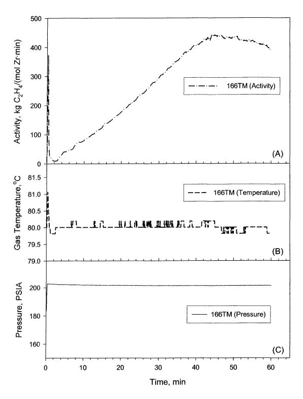
Figure 7.16: Run TM166 using Catalyst TM15 showing (A) activity, (B) gas phase temperature, and (C) pressure profiles.
