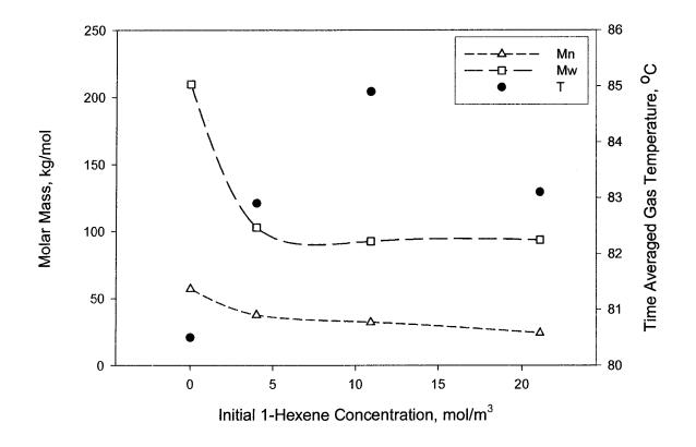
Figure 7.4: Effect of varying initial concentration of 1-hexene on PE molar masses, Mn and Mw, and time averaged gas phase temperature, T.
