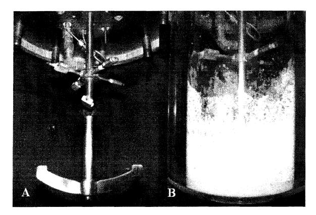
Figure 3.4: Photographs of (A) the impeller system and (B) impellers in action inside Plexiglas replica of reactor.
