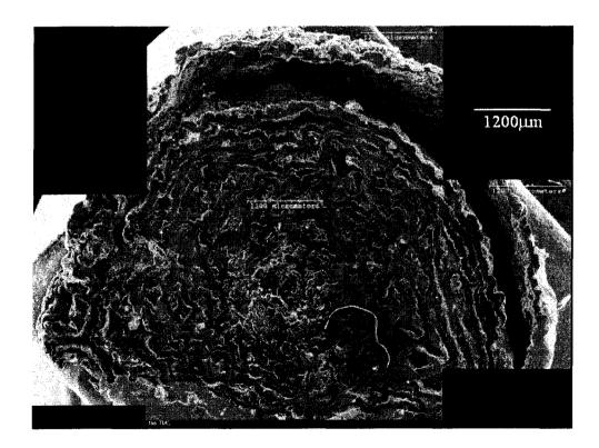
Figure 7.17: Image of a typical cut polymer particle from Run TM166 formed by superimposition of 4 SEM images.
