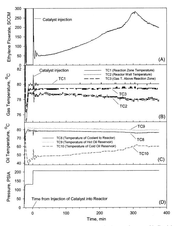
Figure 3.5: Data gathered during a typical polymerization run shown graphically giving (A) ethylene flowrate into reactor, (B) temperature at different locations in the reactor, (C) circulating coolant oil temperature at different locations, and (D) reactor gas pressure.
