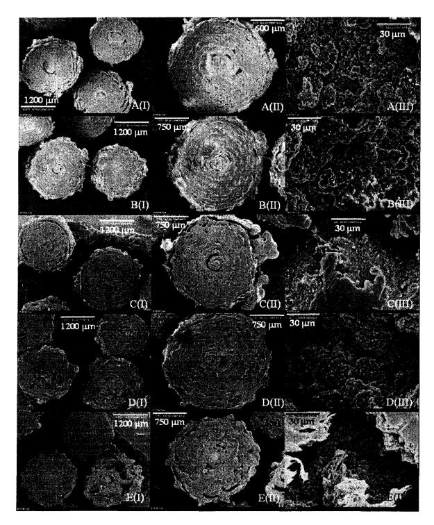
Figure 5.17: SEM images of polymer particles showing effect of gas phase pressure on inner morphologies at (A) 0.70 MPa (Run # 74TM), (B) 1.05 MPa (Run # 76TM), (C) 1.39 MPa (Run # 78TM), (D) 1.74 MPa (Run # 77TM), and (E) 2.06 MPa (Run # 75TM) produced by polymerization at 80°C using Catalyst TM10.
