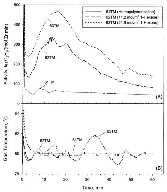
Figure 7.1: Effect of varying initial concentration of 1-hexene on polymerization using Catalyst TM08 showing (A) the activity profiles, and (B) the corresponding gas phase temperature profiles
