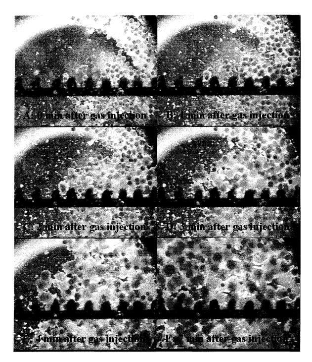
Figure 6.2: Growth of Catalyst TM22 (300-350 µm support size range) particles and fragments during polymerization from (A) immediately after gas entry into micro-reactor to (F) 7 minutes later. Black scale markings are approximately 1 mm apart.
