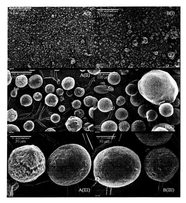
Figure 8.2: SEM images of polymer particles from (A) ethylene homopolymerization run 146TM and (B) ethylene/1-hexene copolymerization run 147TM using Catalyst TM14 taken at low (I) to high (III) magnifications.
