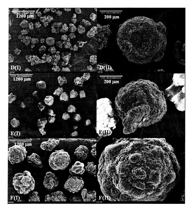
Figure 6.3: (continued from last page) SEM of copolymerization of Catalyst TM20 at low
