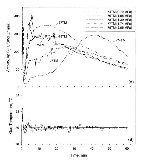
Figure 5.15: Effect of ethylene pressure on gas phase copolymerization using Catalyst TM10 showing (A) activity profiles, and (B) temperature profiles.
