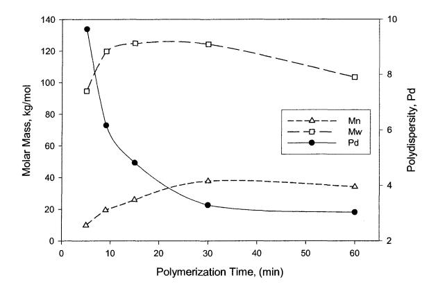
Figure 7.14: Effect of polymerization time on molar masses and polydispersity of copolymers catalyzed by Catalyst TM12 at 80°C.
