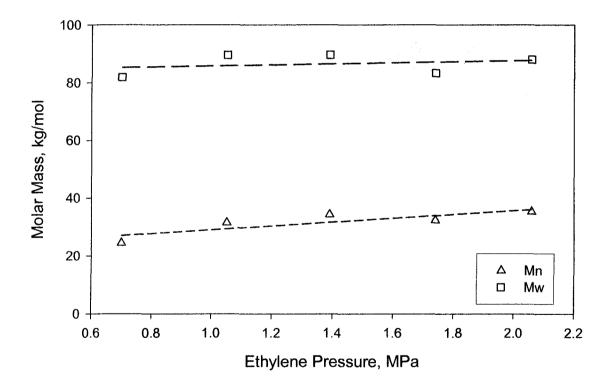
Figure 5.18: Effect of ethylene concentration on product polymer molar masses.
