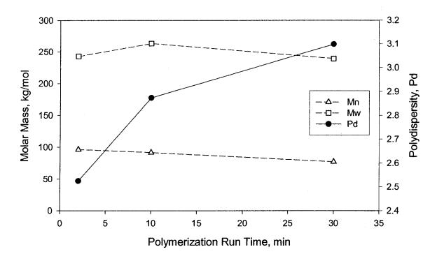
Figure 6.18: Development of molar masses and polydispersities with time during ethylene homopolymerization at 80°C using Catalyst TM22.
