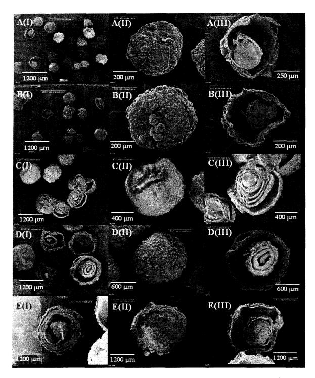
Figure 6.9: SEM of polymer particles produced by copolymerization at  $80^{\circ}$ C with Catalyst TM22 for (A) 2 minutes, (B) 4 minutes, (C) 10 minutes, (D) 15 minutes, and (E) 60 minutes at low (I) and high magnification showing whole (II) and cut (III) particles.
