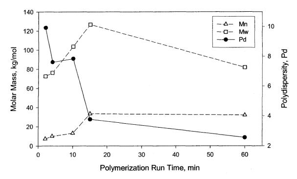
Figure 6.13: Development of molar masses and polydispersities with time during ethylene/1-hexene copolymerization at 80°C using Catalyst TM22.
