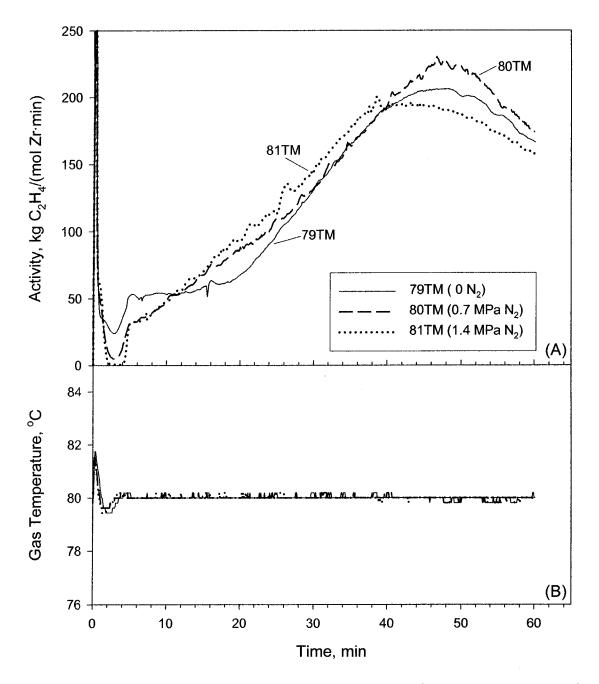
Figure 5.19: Effect of presence of nitrogen on gas phase copolymerization using Catalyst TM10 showing (A) activity profiles, and (B) temperature profiles.
