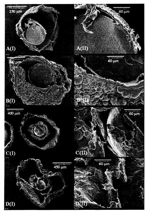
Figure 6.11: SEM showing formation of shells by catalyst/polymer breaking away from surface of catalyst core after (A) 2 min, (B) 4 minutes, (C) 10 minutes, and (D) 15 minutes of copolymerization at 80°C with Catalyst TM22.
