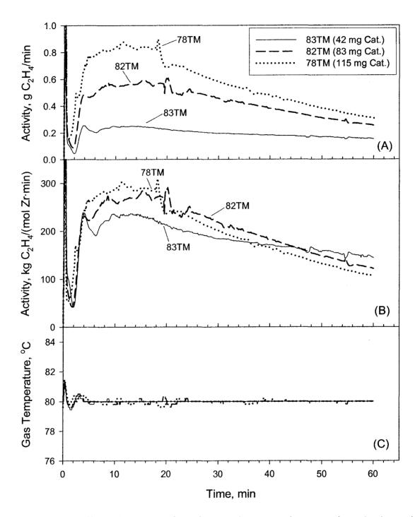
Figure 5.20: Effect of amount of catalyst used on gas phase copolymerization using Catalyst TM10 showing (A) activity profiles, (B) activity profiles per mole of zirconium, and (C) temperature profiles with PID temperature controller switched on.
