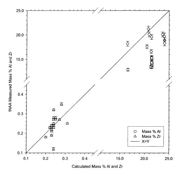
Figure 4.5: Plot of measured Al and Zr concentration versus estimated Al and Zr concentration in prepared catalysts.
