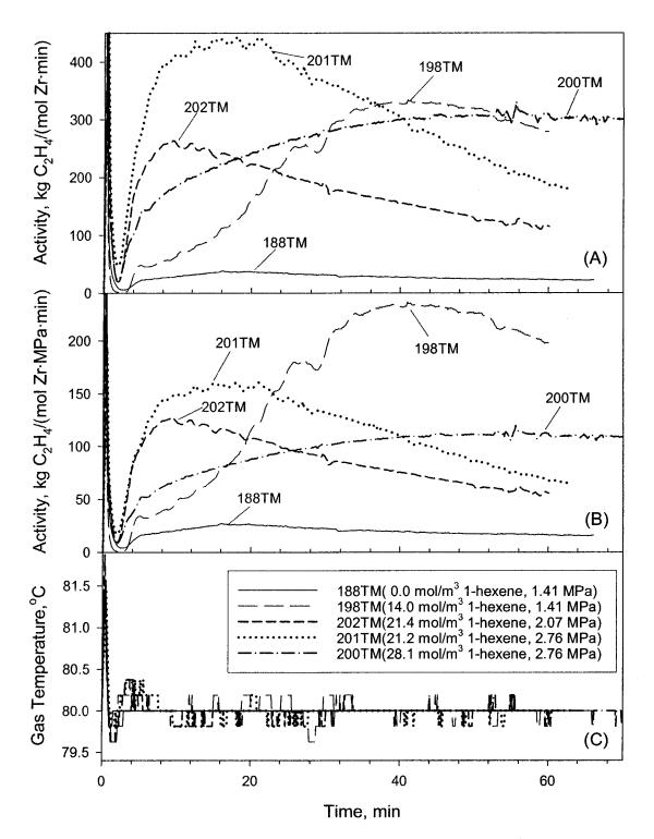
Figure 7.6: Effect of varying initial concentration of 1-hexene and ethylene pressure on polymerization using Catalyst TM17 showing (A) activity profiles, (B) activity profiles normalized with respect to total pressure, and (C) gas phase temperature profiles.
