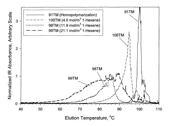
Figure 7.12: TREF profiles of homopolymer and copolymers formed from different initial concentration of 1-hexene.
