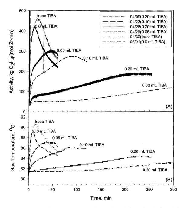
Figure 5.6: Effect of TIBA on gas phase homopolymerization using Catalyst TM02 showing (A) activity profiles, and (B) temperature profiles.
