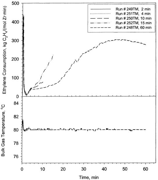
Figure 6.7: Activity and bulk gas temperature profiles of copolymerization of ethylene and 1-hexene with Catalyst TM22 at 80°C
