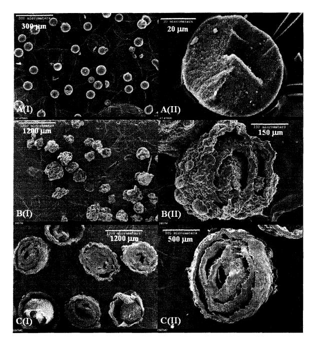
Figure 6.5: SEM of development of internal structure of particles during copolymerization with (A) Catalyst TM20 at 80°C after (B) 10 minutes, and (C) 60 minutes taken at low (I) and high (II) magnification.
