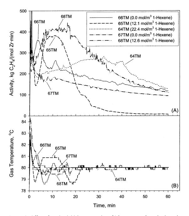
Figure 7.2: Effect of varying initial concentration of 1-hexene on polymerization using Catalyst TM08 showing (A) the activity profiles, and (B) the corresponding gas phase temperature profiles after coolant reservoir modification.
