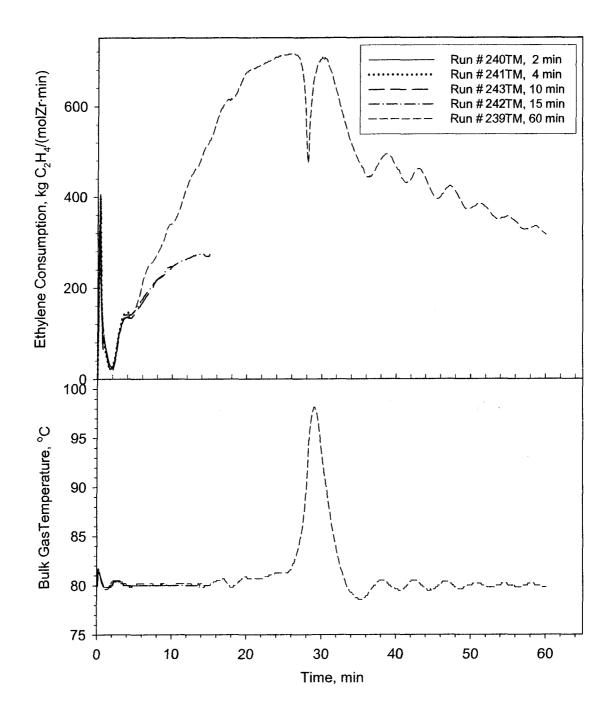
Figure 6.4: Activity and bulk gas temperature profiles of copolymerization of ethylene and 1-hexene at 80°C for runs of various lengths using Catalyst TM20
