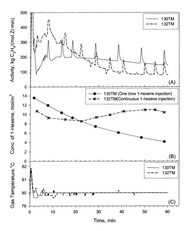
Figure 7.8: Experiments to study variation of concentration of 1-hexene during polymerization using Catalyst TM13 at 80°C showing (A) activity profiles, (B) gas phase concentration of 1-hexene, and (C) gas phase temperature profiles.
