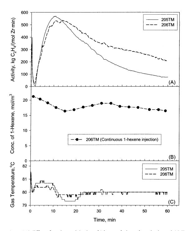
Figure 7.10: Effect of continuous injection of 1-hexene during polymerization at 2.1 MPa using Catalyst TM17 at 80°C showing (A) activity profiles, (B) concentration of 1-hexene, and (C) temperature profiles.
