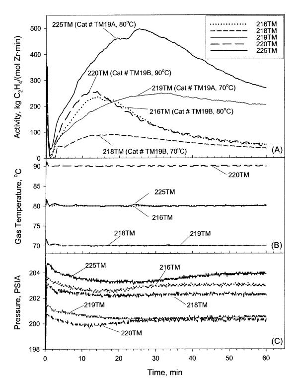
Figure 8.5: Effect of temperature on polymerization runs with different size catalysts showing (A) activity, (B) gas phase temperature, and (C) pressure profiles.
