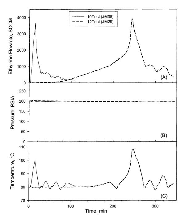
Figure 5.2: Effect of high activity on reaction profiles. Polymerization data from test runs using Catalysts JM38 and JM29 showing (A) rate of ethylene flow into reactor, (B) reactor gas pressure, and (C) gas temperature.
