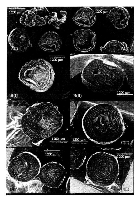
Figure 5.13: SEM images of polymer particles showing effect of gas phase polymerization temperature on inner morphologies at (A)  $60^{\circ}$ C (Run # 197TM), (B)  $80^{\circ}$ C (Run # 192TM), (C)  $90^{\circ}$ C (Run # 194TM), and (D)  $100^{\circ}$ C (Run # 196TM) using Catalyst TM17.
