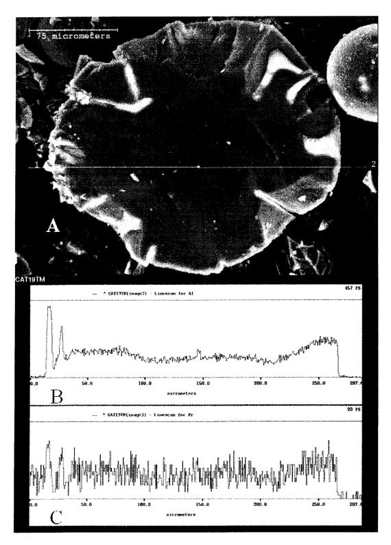
Figure 4.3: (A) Cut TM19B particle for determining distribution of metal showing linescanning position; (B) EDX linescan for aluminum; (C) EDX linescan for zirconium
