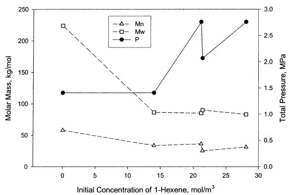
Figure 7.7: Effect of varying initial concentration of 1-hexene and ethylene pressure on PE molar masses, Mn and Mw during polymerization at 80°C using Catalyst TM17.
