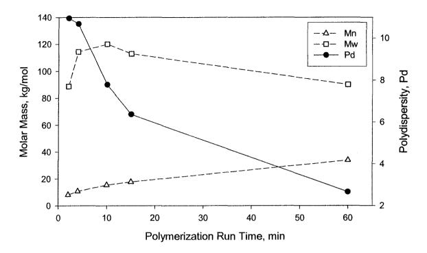
Figure 6.6: Development of molar masses and polydispersities with time during ethylene/1-hexene copolymerization at 80°C using Catalyst TM20.
