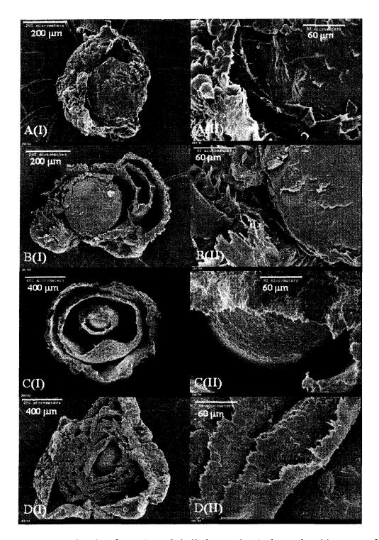
Figure 6.12: SEM showing formation of shells by catalyst/polymer breaking away from surface of catalyst core after (A) 2 min, (B) 4 minutes, (C) 10 minutes, and (D) 15 minutes of copolymerization at 70°C with Catalyst TM22.
