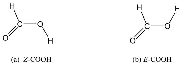
Figure 4.S1. The two observed conformations of formic acid, showing the nomenclature adopted. (a) is the Z -conformer, also named as synperiplanar where the dihedral angle H-C-O-H is 0^\circ . (b) is the E -conformer, also named as antiperiplanar where the dihedral angle H-C-O-H is 180^\circ .
