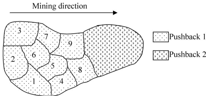
Figure 4.2: Schematic representation of an oil sands deposit showing mining-cuts and pushbacks
