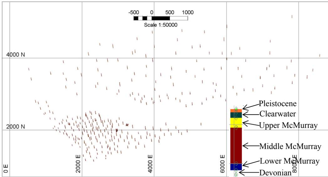
Figure 5.21: A 2D projection of 326 drillholes used for resource modeling and a drillhole cross section
