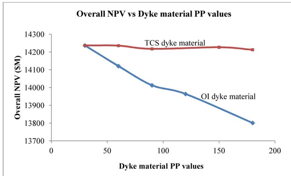
Figure 5.13: General trend of overall NPV with PP values of dyke material
