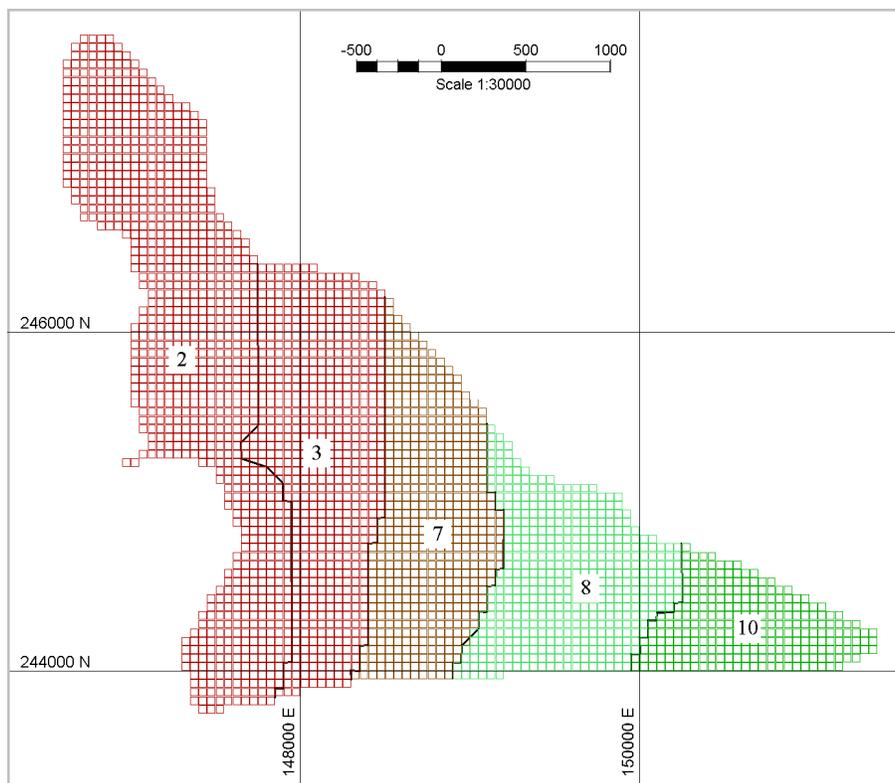
Figure 5.14: Mining sequence at level 305m with a west-east mining direction
