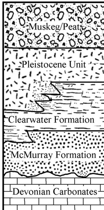
Figure 2.1: Sketch of the vertical soil profile of an oil sands formation modified after Dusseault (1977)
