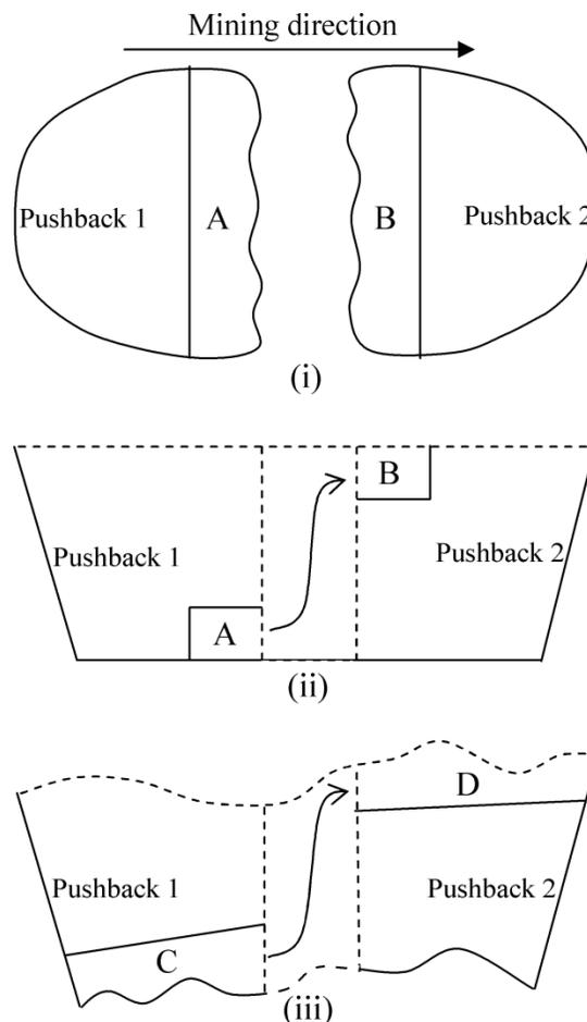
Figure 4.3: Developing pushback mining precedence constraints: (i) Plan view and (ii) Cross sectional view; of final pit with flat topography and bottom showing pushbacks 1 and 2 and the sets of bounding mining-panels (iii) Cross sectional view of final pit with undulating topography and bottom showing pushbacks 1 and 2 and the sets of bounding mining-panels
