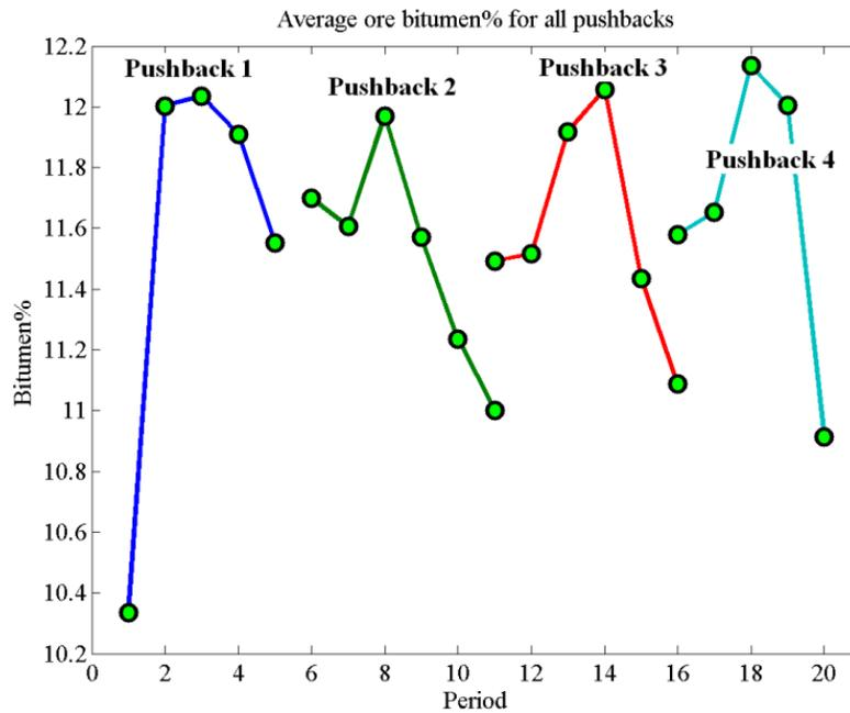
Figure 5.10: Average ore bitumen grade for all pushbacks
