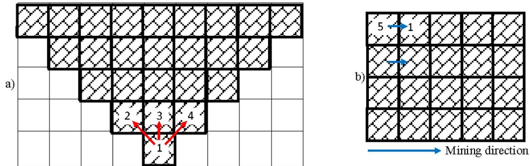
Figure 4.1: Mining-panels extraction precedence in the MILGP formulation modified after Ben-Auwah and Askari-Nasab (2011): a) cross sectional view and b) plan view
