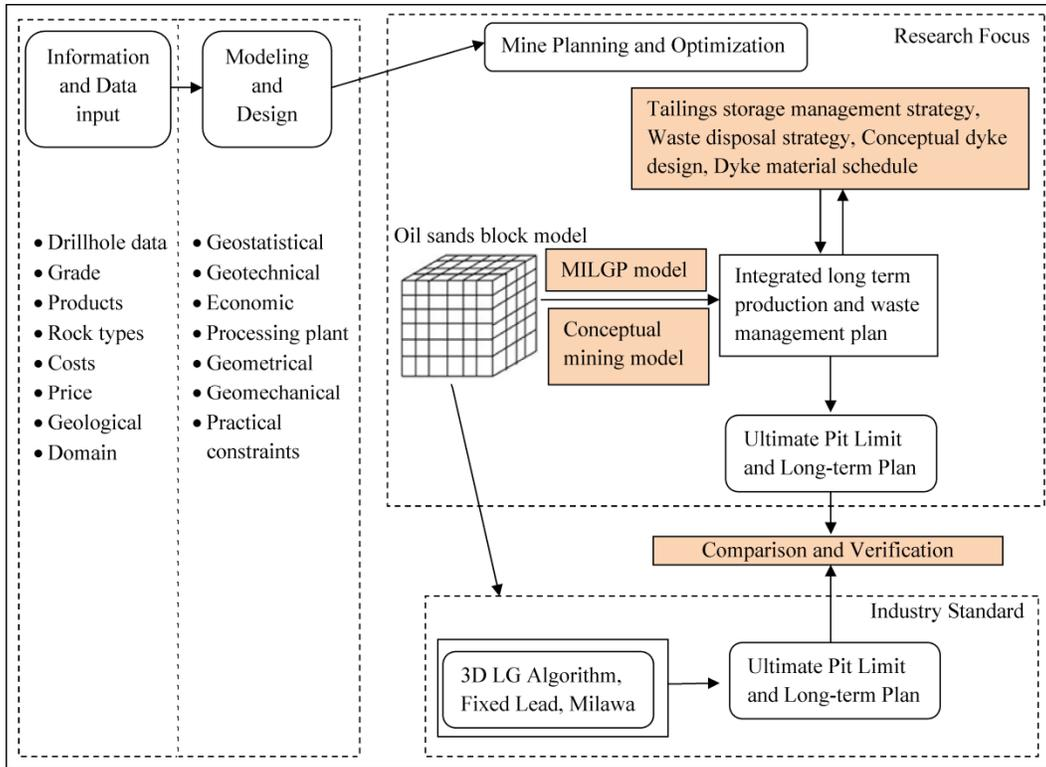
Figure 5.1: General workflow of experimentation methodology
