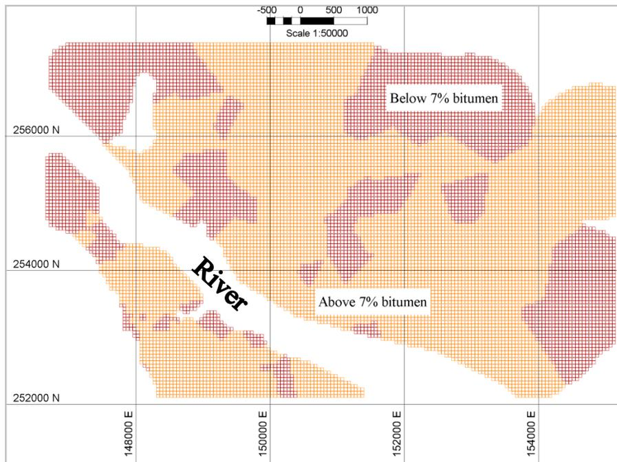
Figure 5.22: General bitumen content distribution in study area on level 305m
