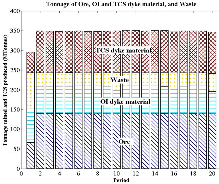
Figure 5.6: Schedules for ore, OI and TCS dyke material, and waste tonnages produced over 20 periods
