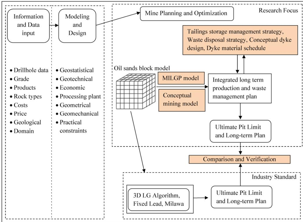
Figure 5.1: General workflow of experimentation methodology
