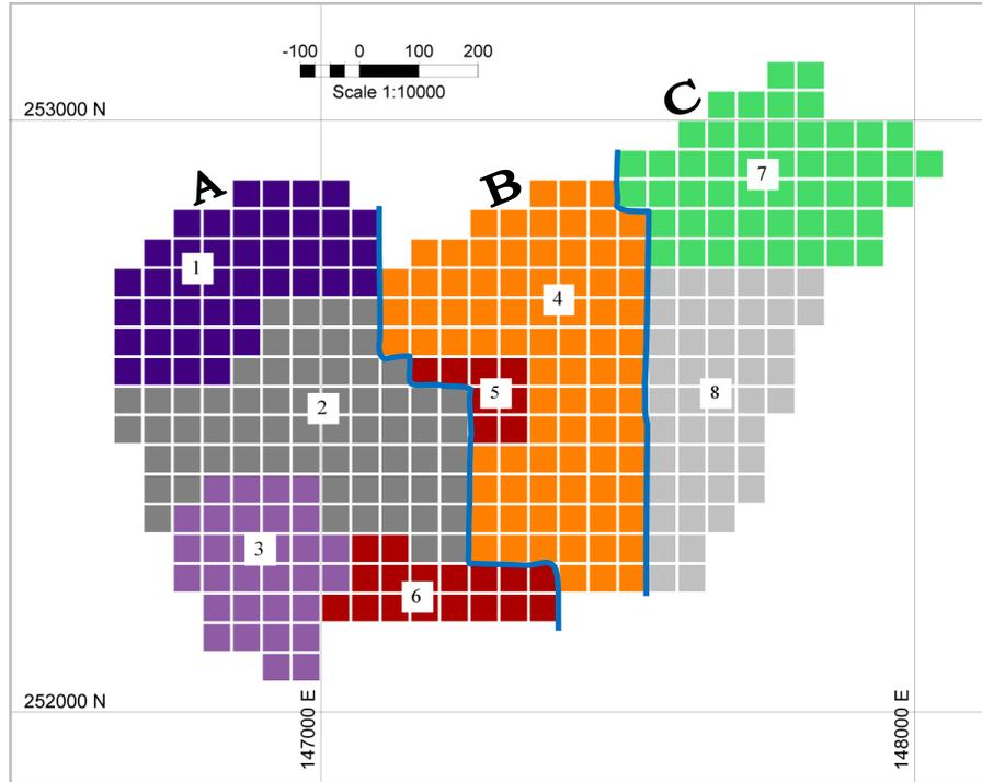
Figure 2.3: 8 Mining-cuts of blocks from hierarchical clustering, and 3 mining-panels
