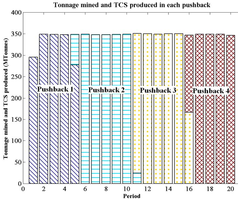
Figure 5.7: Material mined and TCS dyke material tonnage produced in each pushback for 20 periods
