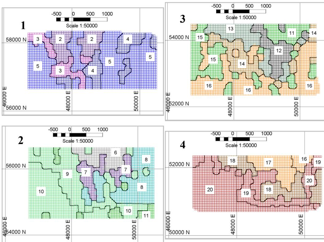
Figure 5.5: Pushbacks 1, 2, 3 and 4 mining sequence at level 325 m
