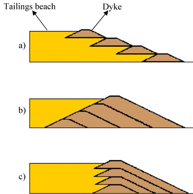
Figure 2.2: a) Upstream construction, b) downstream construction, and c) centerline construction (after Vick, 1983)
