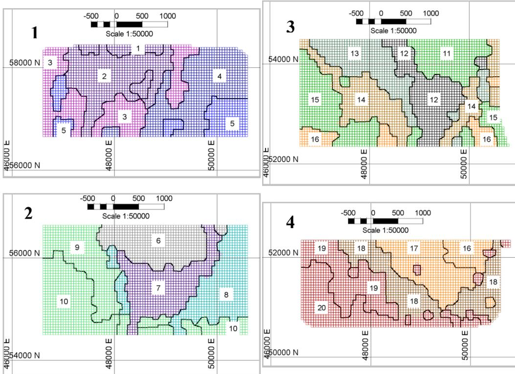
Figure 5.4: Pushbacks 1, 2, 3 and 4 mining sequence at level 310 m
