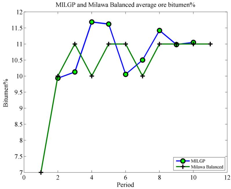
Figure 5.39: MILGP model and Whittle Milawa Balanced average ore bitumen
