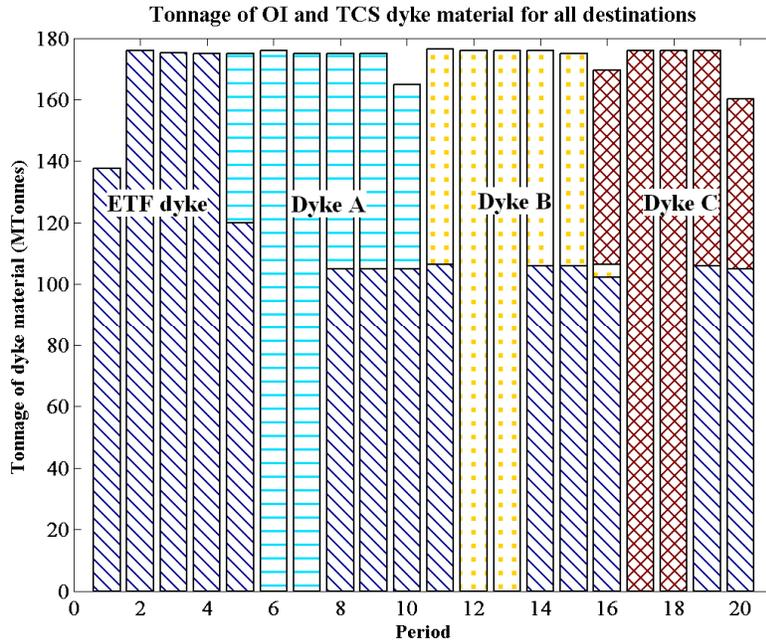
Figure 5.8: Dyke material tonnage sent to the various dyke construction destinations for 20 periods
