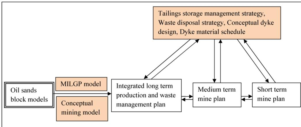
Figure 3.1: The MILGP model framework environment and interactions
