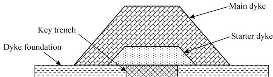
Figure 3.3: Schematic diagram showing cross section of a dyke
