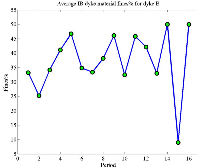
Figure 5.31: Average IB dyke material fines percent for dyke 'B' in all periods
