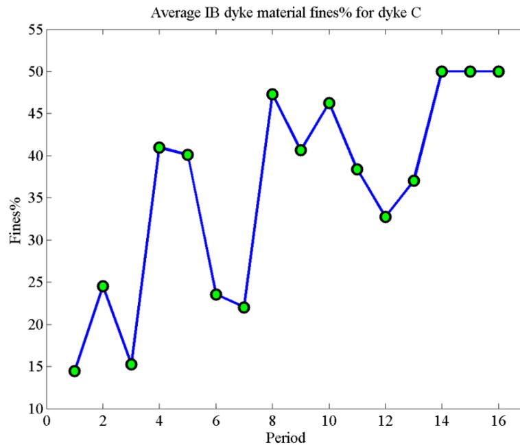
Figure 5.32: Average IB dyke material fines percent for dyke 'C' in all periods
