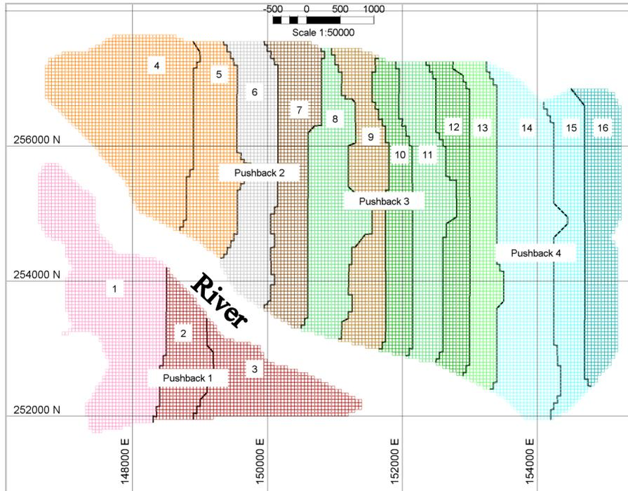
Figure 5.25: Mining sequence at level 305m for all pushbacks with a west-east mining direction
