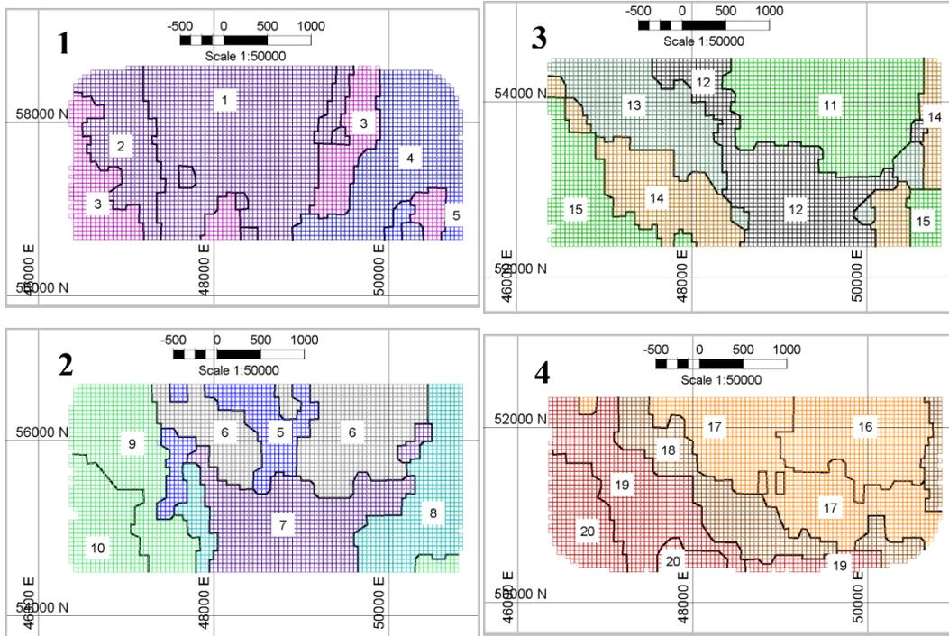
Figure 5.2: Pushbacks 1, 2, 3 and 4 mining sequence at level 280 m
