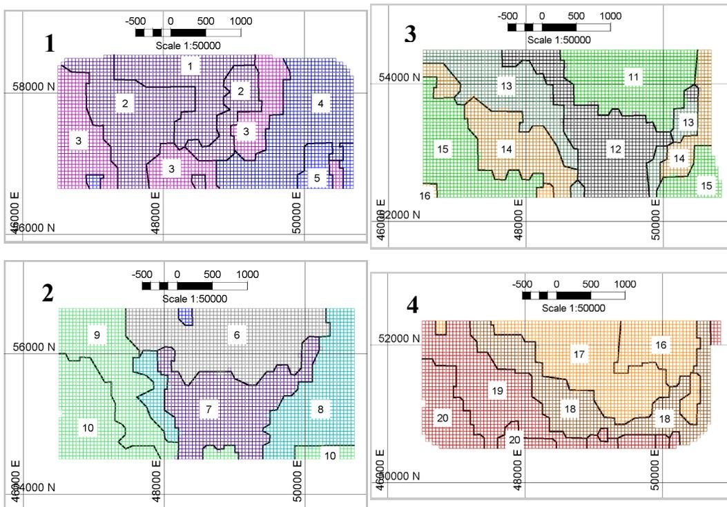
Figure 5.3: Pushbacks 1, 2, 3 and 4 mining sequence at level 295 m
