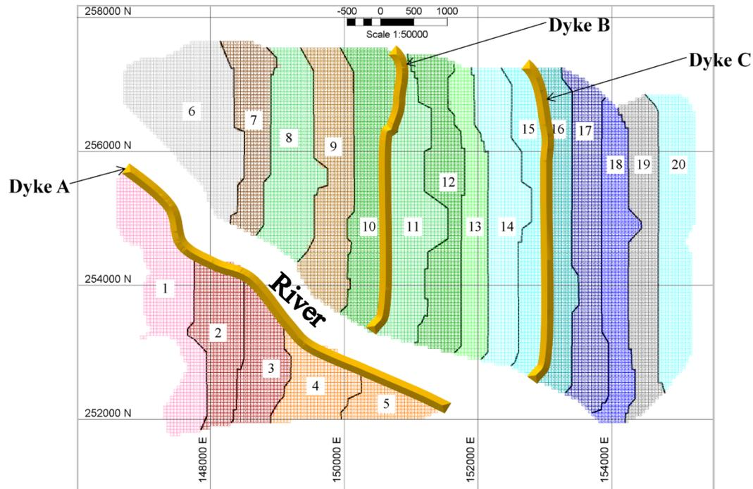
Figure 5.23: Mining-panels and in-pit dyke locations at level 305m
