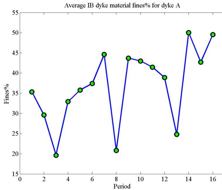
Figure 5.30: Average IB dyke material fines percent for dyke 'A' in all periods
