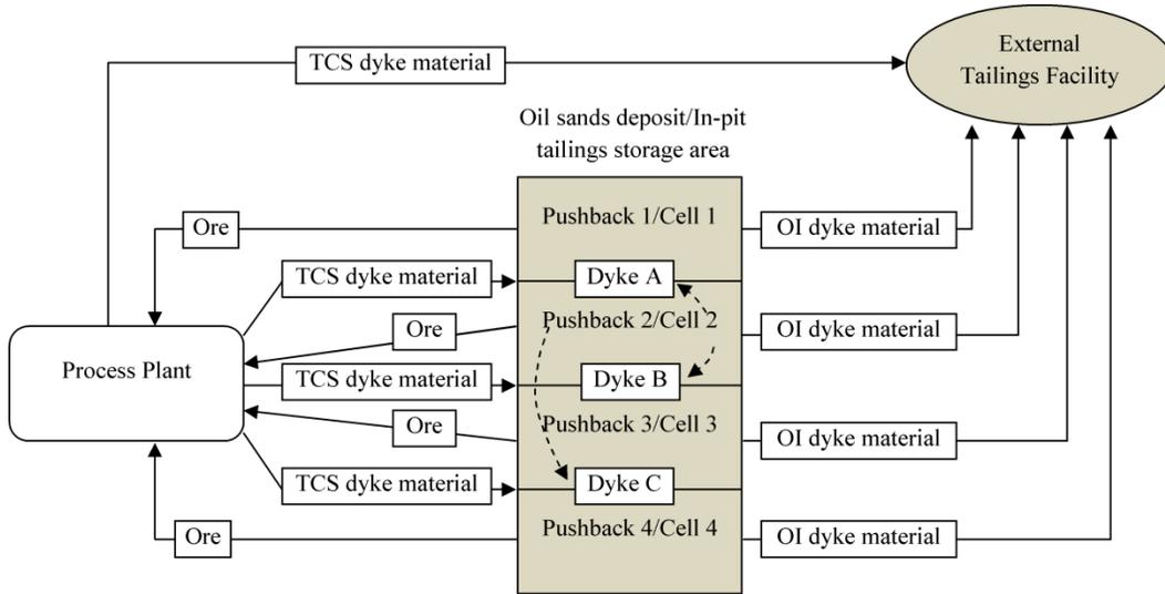
Figure 3.2: Conceptual mining model showing mining and waste management strategy modified after Askari-Nasab and Ben-Awuah (2011)
