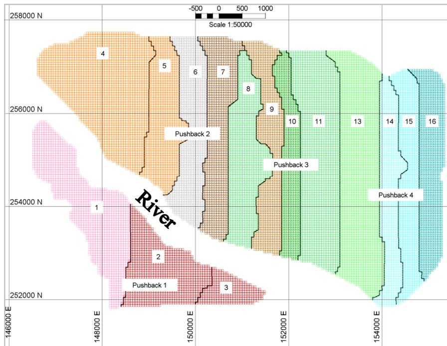
Figure 5.24: Mining sequence at level 320m for all pushbacks with a west-east mining direction
