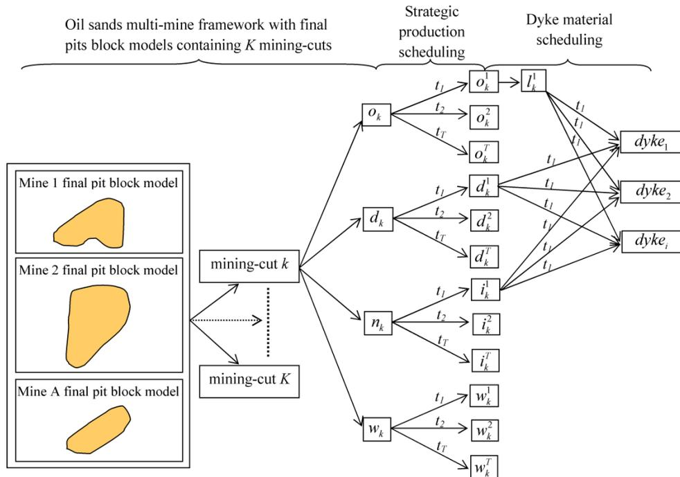
Figure 1.1: Schematic representation of the problem definition showing strategic production and dyke material scheduling modified after Ben-Awuah and Askari-Nasab (2011)
