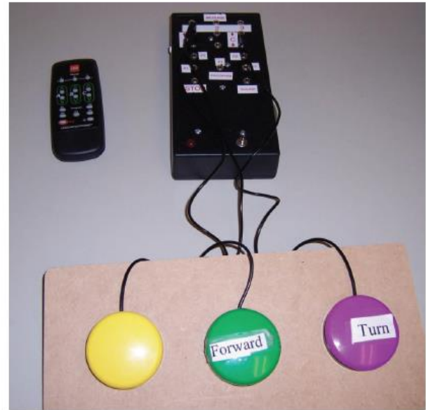
Figure 2. Lego Mindstorms remote controller (left), adapted controller with switches (right).
