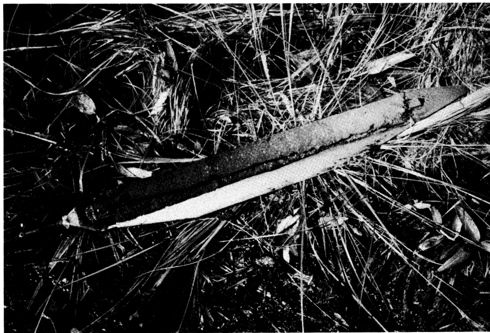
Photograph 2.10 Illustration of a Macauley sampler with a peat core.
