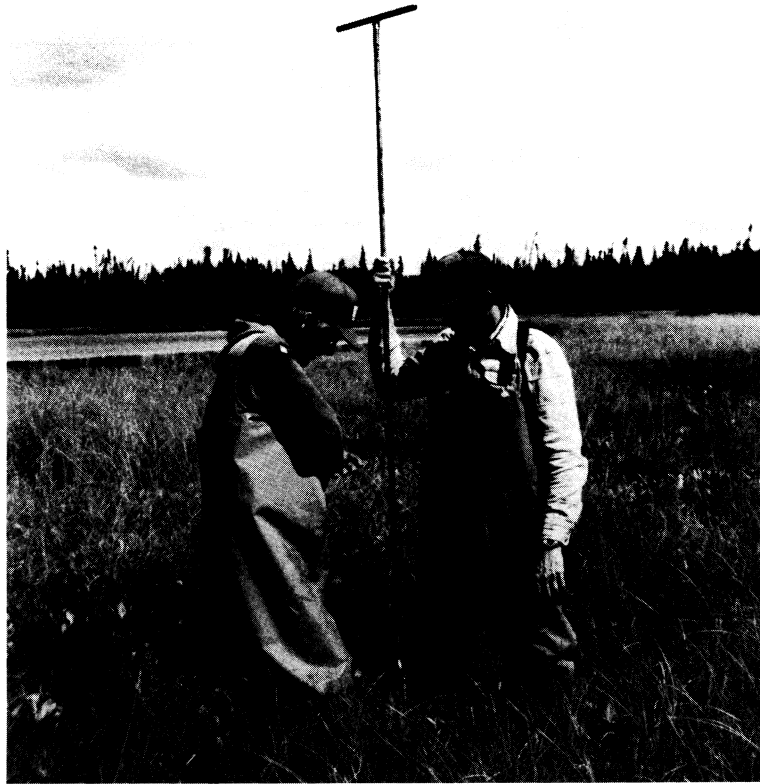
Photograph 2.9 Macauley peat sampler being used in a natural peatland.
