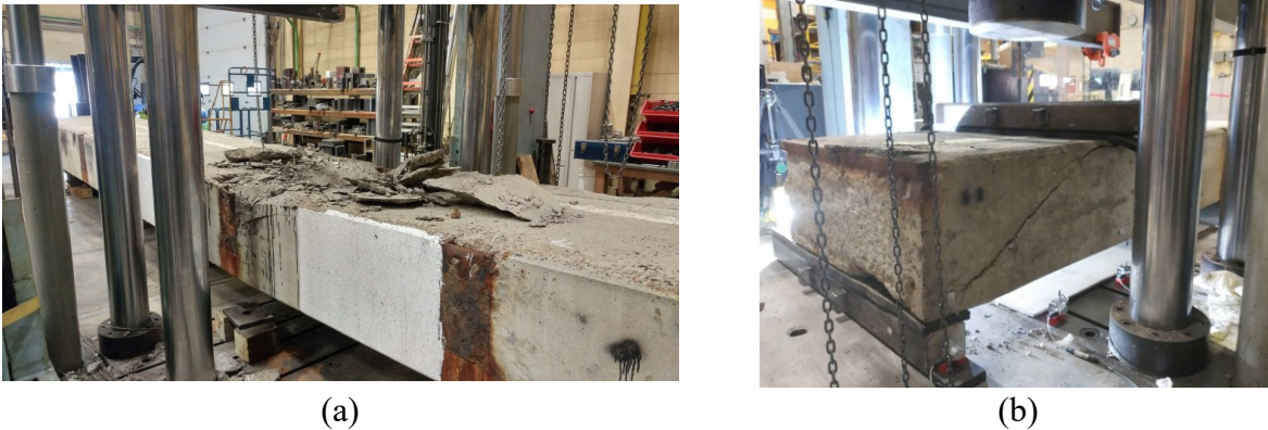
Figure 3-9: Failure of the tested PC girder: (a) flexure test showing concrete crushing, and (b) shear test showing diagonal tension failure
