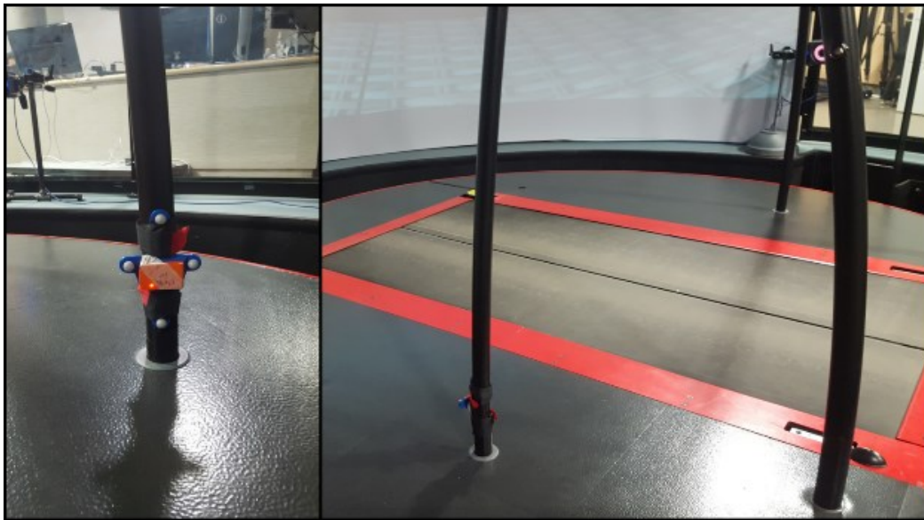
Figure 4.7: Location of the rigid plate and markers for tracking platform motion. This cluster was placed on the frame, rather than directly on the surface of the platform, to avoid the possibility of a participant stepping on it during the step-to-target task.
