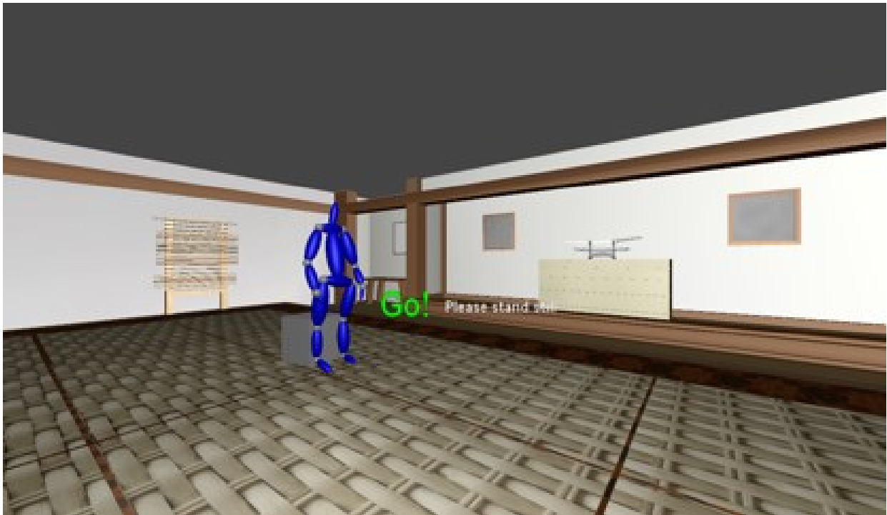
Figure 4.2: Virtual environment for the calibration routine. Tasks included sit-to-stand, heel-to-toe shift (eyes open and closed), and a staggered stance (left foot in front of right, and vice versa). The purpose of this calibration routine was to obtain accurate three-dimensional joint angles that are not affected by marker cluster plate placement.
