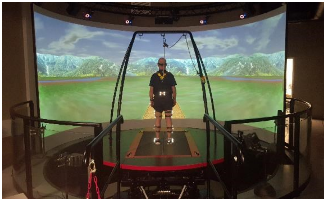
Figure 4.5: A participant on the CAREN prior to the simulated rocky surface walking task. Participants wore a full-body safety harness that was secured to the fixed, overhead frame. The length of the harness was adjusted separately according to the requirements of each task within the protocol. In case of a critical loss of balance or a fall, the CAREN's emergency stop was in place to immediately cease all functions.
