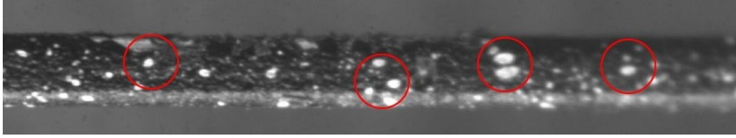
Figure C.3. Archwire speckling with white acrylic paint. Inconsistencies in speckle size are highlighted in circled regions.
