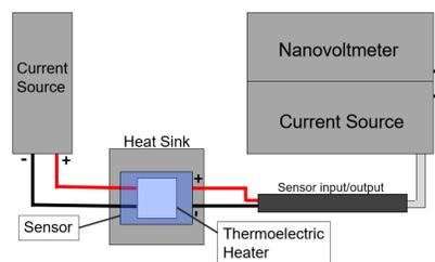
Figure 3: Schematic of the experimental setup used for collecting data from the temperature sensors
