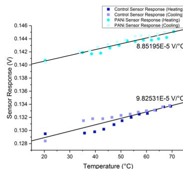
Figure 8: Sensor response as a function of temperature for both the control and PANi sensors with sensitivities through a heating and cooling cycle at 0.29mA.
