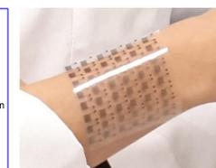
Figure 12: Demonstration of tattoo temperature sensors for wearable applications
