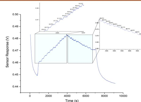
Figure 10: Control sensor response as a function of time through a timed heating and cooling cycle at 1.0mA. Areas of the graph are enlarged to show detail.
