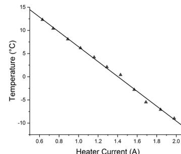
Figure 5: Heater temperature as a function of heater current at low temperatures. Heater temperature is measured by a thermocouple.
