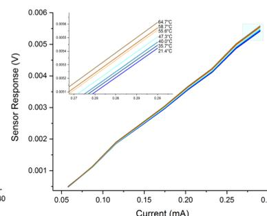
Figure 7: PANi Sensor response as a function of current through a heating cycle. An area of the graph is enlarged to show details of the plot.
