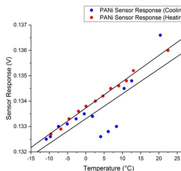
Figure 9: PANi sensor response as a function of temperature through a low temperature heating and cooling cycle at 0.29mA.
