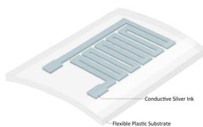
Figure 1: Flexible temperature sensor schematic
