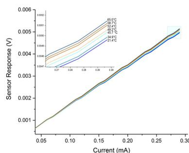
Figure 6: Control Sensor response as a function of current through a heating cycle. An area of the graph is enlarged to show details of the plot.
