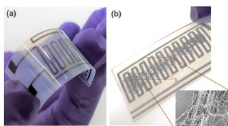
Figure 2: (a) Flexible temperature sensor (b) Temperature sensor modified with PANi nanowires. Inset of Figure 2(b) shows a magnified SEM image of PANi nanowires
