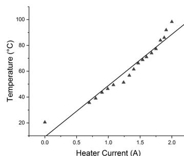
Figure 4: Heater temperature as a function of heater current at increasing temperatures. Heater temperature is measured by a thermocouple.
